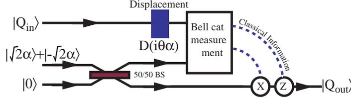
**Figure 1.** Schematics for implementing a rotation around  $Z$ . We begin by first shifting our qubit a small distance out of the computational basis and then using teleportation to project back into the qubit space.
