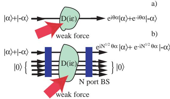
**Figure 4.** Schematic diagram of the action of a weak force causing a displacement  $D(i\epsilon)$  on a Schrödinger cats state  $|\alpha\rangle + |-\alpha\rangle$ . In a) a single mode case is illustrated while in b) an  $N$  mode situation is considered.
