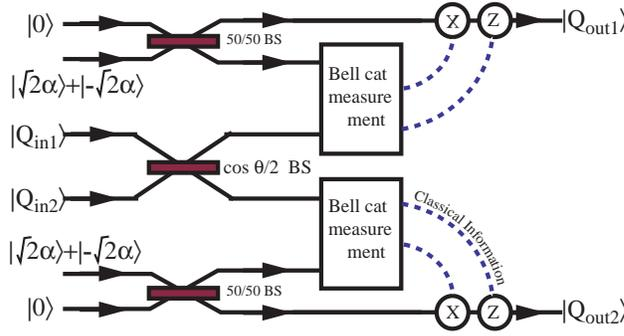
**Figure 3.** Schematics of implementing an entangling gate. For a sufficiently small value of  $\theta^2\alpha^2$  this gate is near deterministic. Repeated application of this gate can build up to a gate locally equivalent to a CNOT gate, with high probability.
