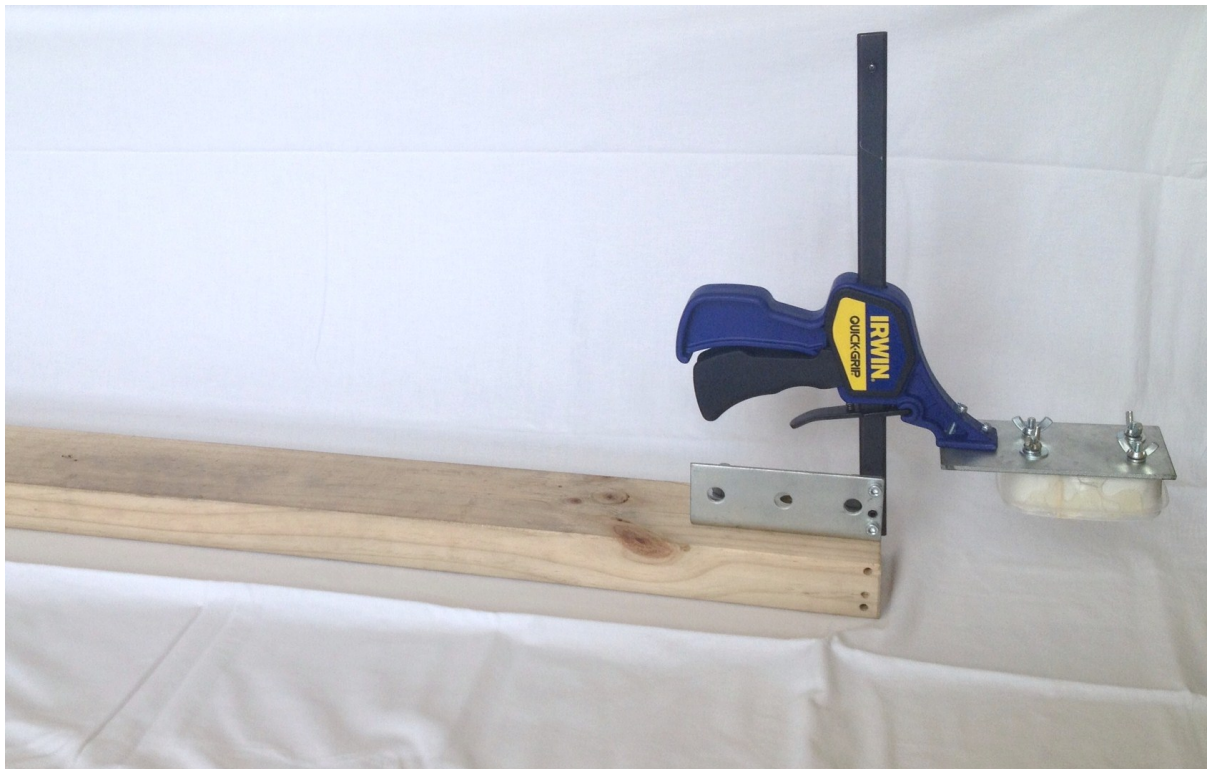
Figure 23. Photo showing the clamping device for the GME and Clam1 testing positions
