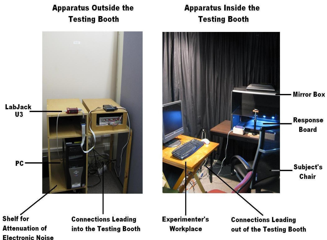
Figure 4. Apparatus outside and inside the testing booth. All electronic equipment producing any kind of noise was placed outside the testing booth. The experimenter's workplace was set up in the booth because it was hoped that the subjects would feel observed and so would put more effort into their performance.
