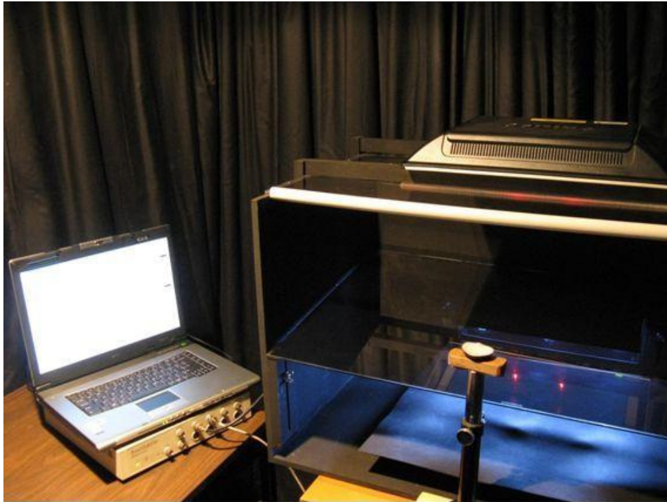
Figure 5. Two-channel voltage impulse recordings from two light-emitting diodes with PowerLab/4SP.
