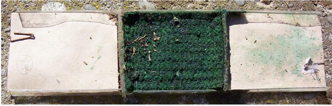
Figure 2. An example BUM board showing central compartment holding dye-soaked sponge and outer compartments holding paper.
