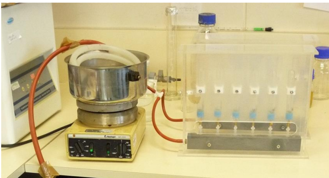
Figure 2.2 Arrangement for heating gas. Nitrogen gas is ducted through red tubing to white silicone tubing immersed in a pan of simmering water. Warmed gas exits through red tubing (connection point not visible) to two inverted sparging manifolds, each holding six tubes.
