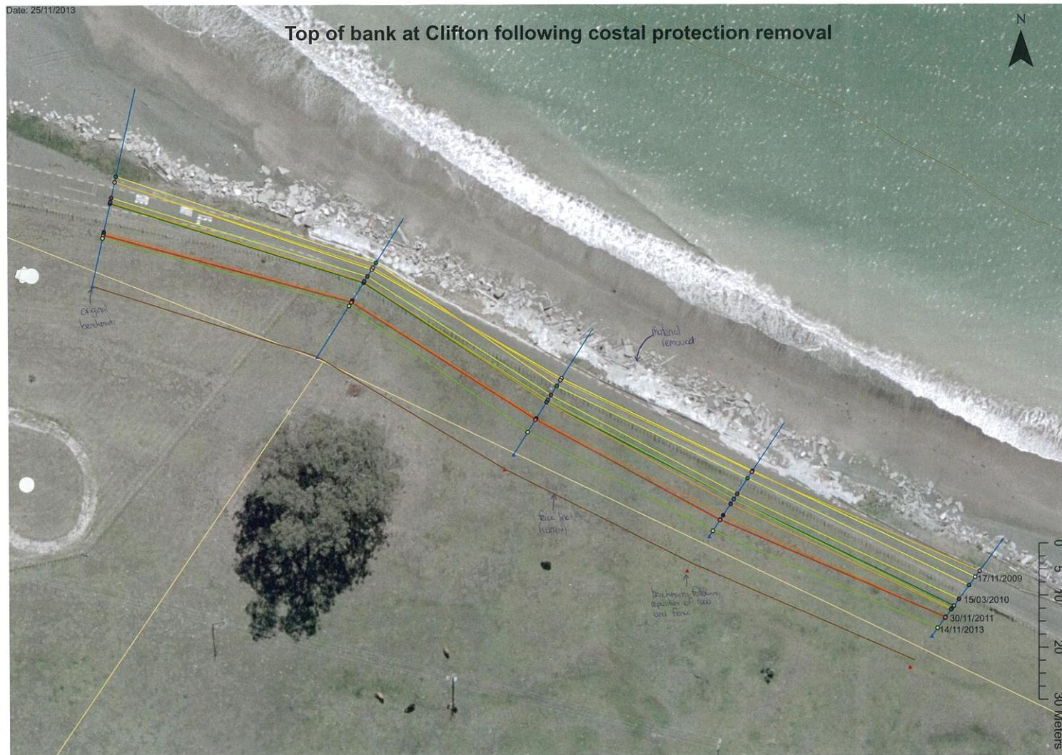
Figure 3 Cross section of coastal erosion on the road to Clifton Camp since protection structures have been removed (Source: Hawke's Bay Regional Council GIS, 2013)
