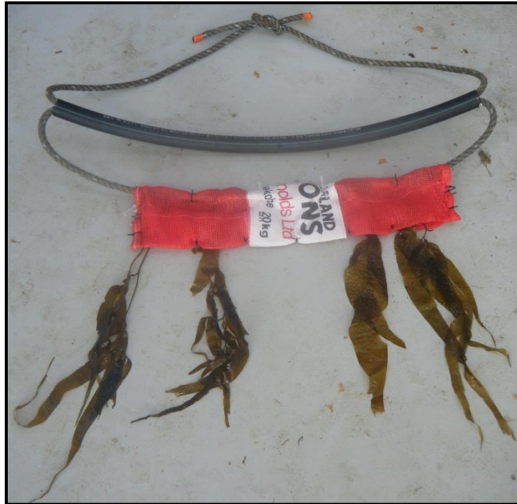
Figure 3.2: M. pyrifera growing frame used to conduct IMTA trials in Big Glory Bay, Stewart Island, New Zealand
