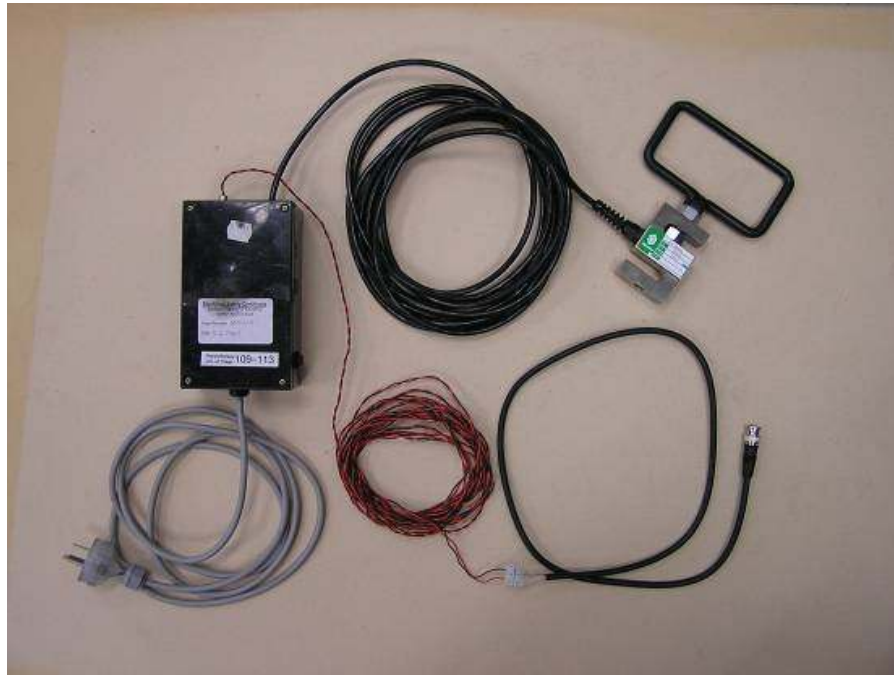
FIGURE 3.4: S- shaped load cell with attached handle and required cables data gathering during catch and drag sequence.
