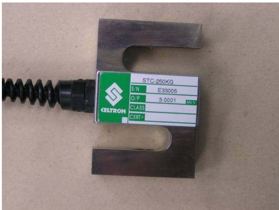
FIGURE 3.2.: S-shaped load cell used to calculate hand forces during catch and drag phase of sheep shearing.
