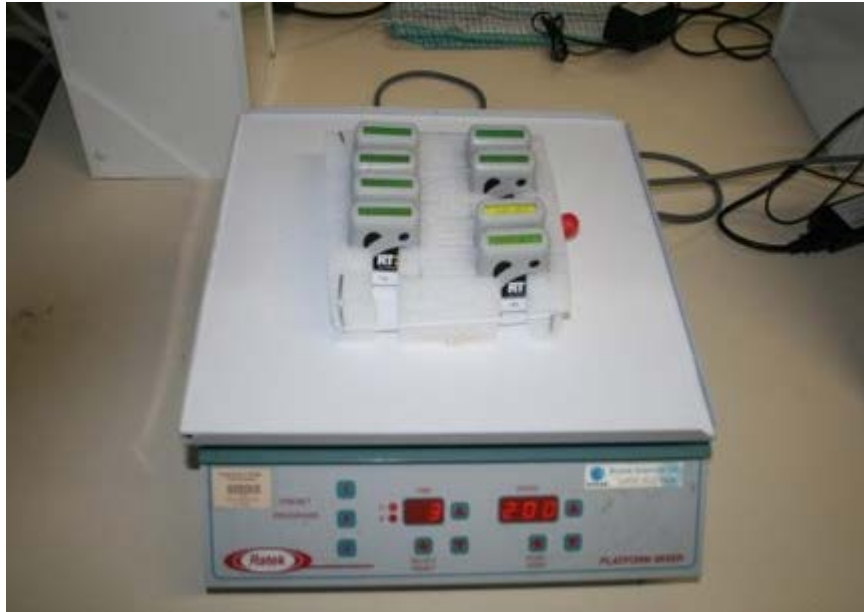
RT3 monitor testing procedure on shaker table
