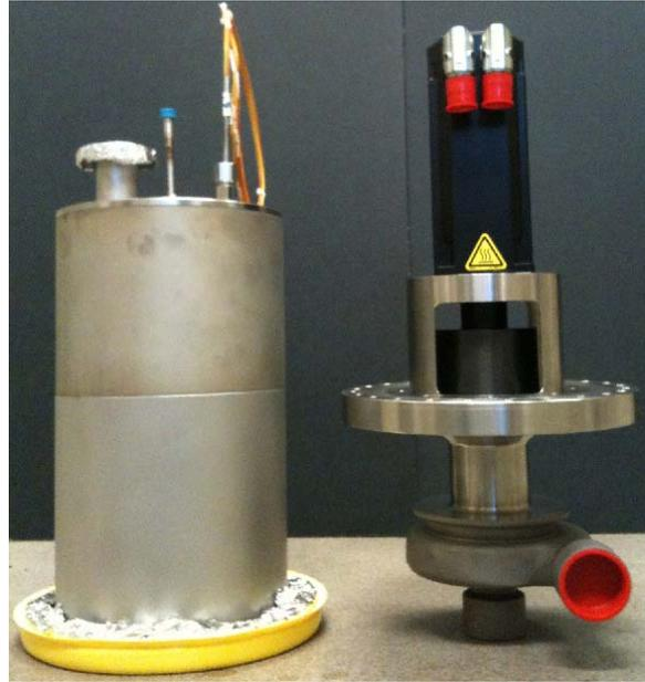
**Figure 3. Mechanical NaK pump prototype.** *Left is the motor can and to the right is the motor- pump.*
