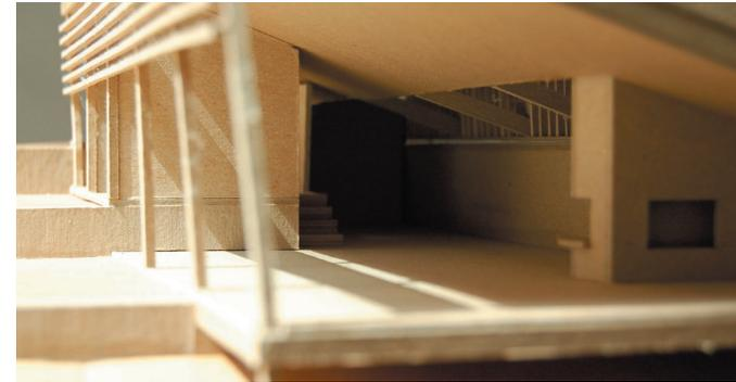
Fig. 143, 144 | Solar study model showing summer shading and winter sunlight penetration
