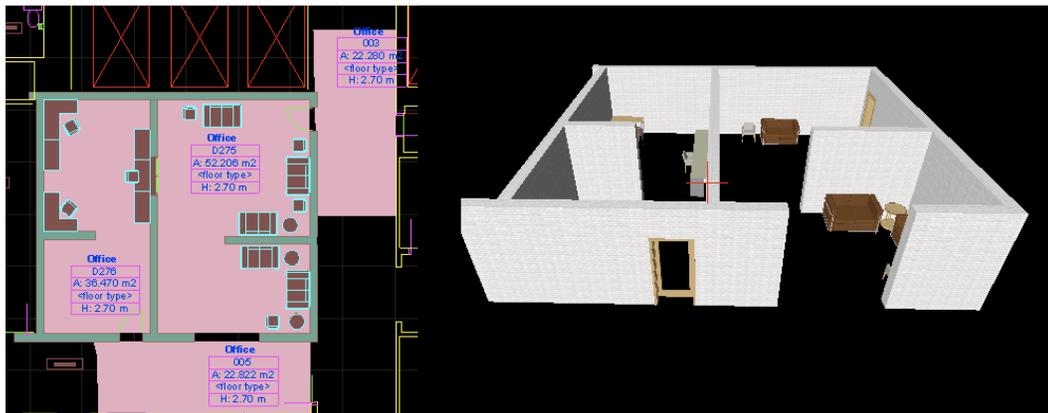
**Figure 3.5: IFC Model of DI Reception in 2-D and 3-D**
