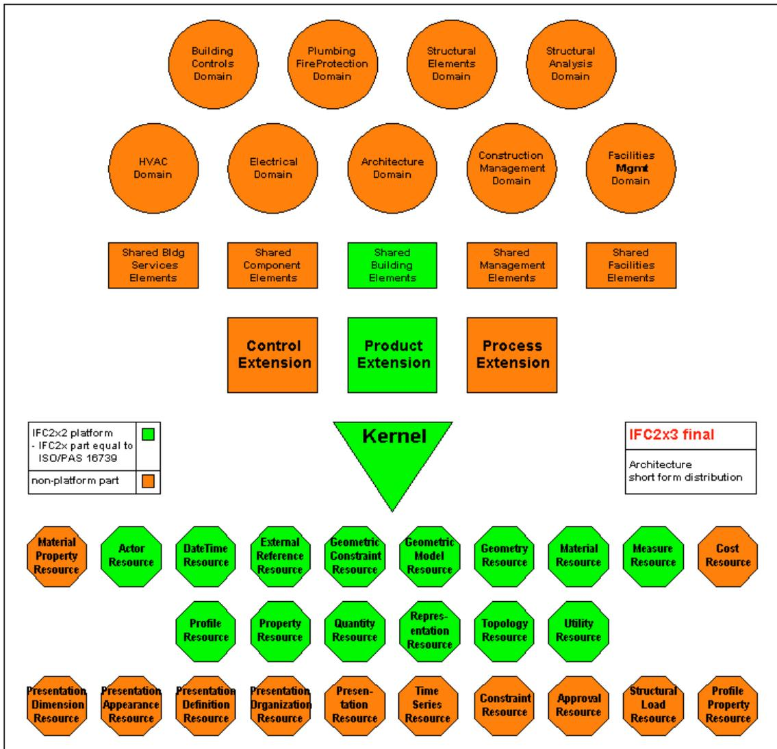
Figure 3.2: IFC Architecture Diagram (IFC Model Guide, 2004)
