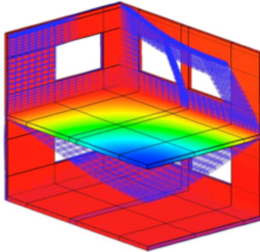
**Figure 3.1: Stress and Displacement Simulation Caused by Vertical Loads (van Treeck et al., 2003)**
