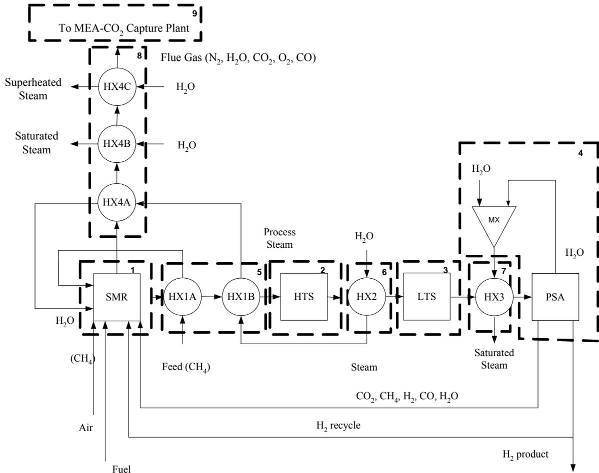
**Figure 3.12: Process flow diagram for the H<sub>2</sub> Plant with MEA-CO<sub>2</sub> capture**
