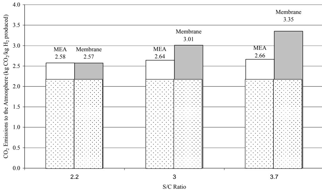
**Figure 4.4: Comparison of CO<sub>2</sub> emissions to the atmosphere:  $T_{SMRin} = 900$  K,
