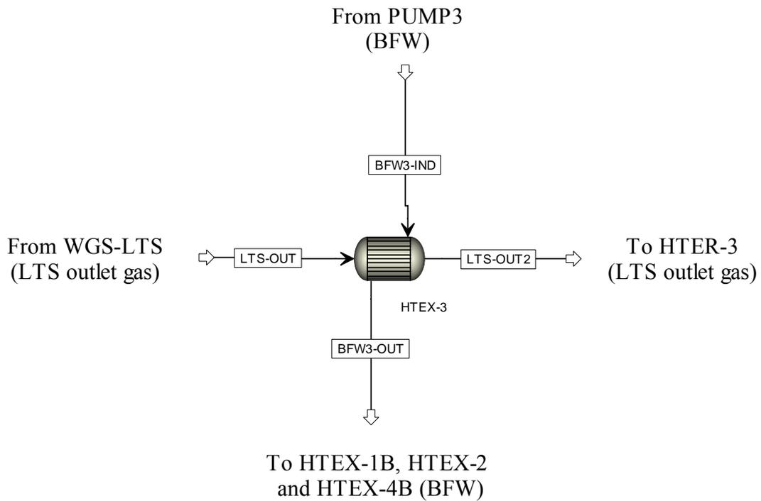
**Figure 3.10: Block # 7 - LTS heat exchange system**
