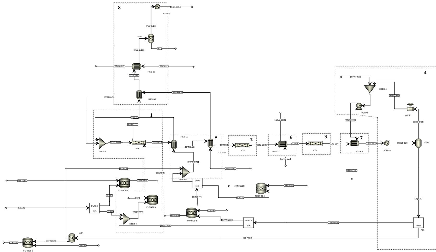
Figure 3.2: Aspen flowsheet for H<sub>2</sub> plant without CO<sub>2</sub> capture
