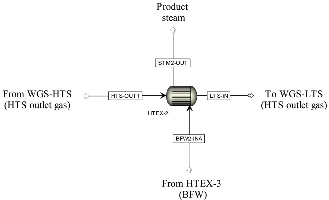
**Figure 3.9: Block # 6 - HTS heat exchange system**
