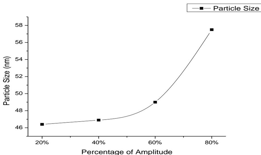
Figure 16. Change of Particle Size with Percentage of Amplitude of Combined Emulsifying Method of Probe Ultrasound + Bath Ultrasound
