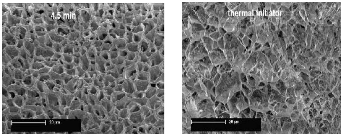
Figure 7. SEM image of ultrasound initiated Dex-MA hydrogels with polymerization time of 4.5min, compared to thermal initiation hydrogels (Cass et al., 2010)
