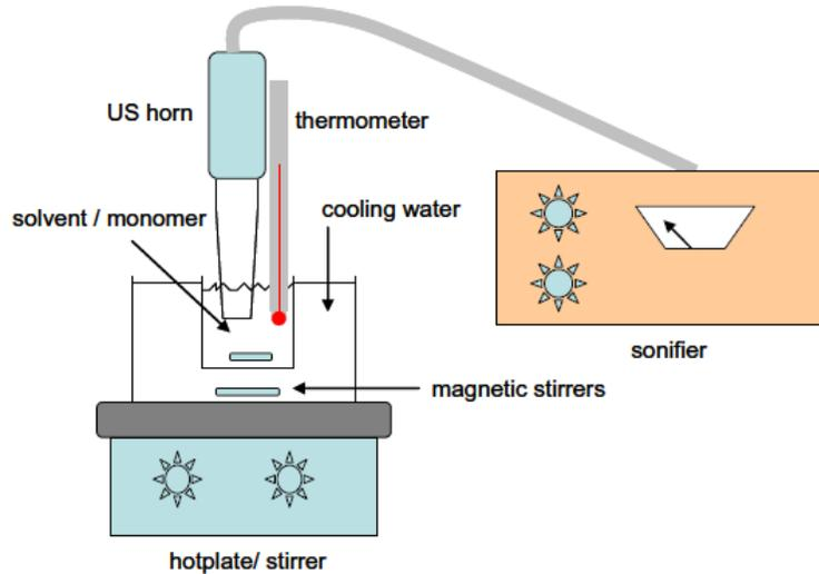
Figure 6. Set-up diagram of ultrasound device applied for hydrogels preparation (Cass et al., 2010)
