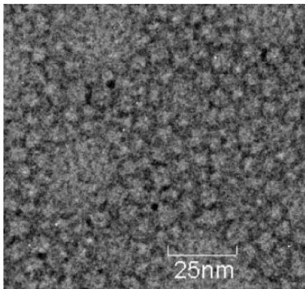
Figure 1. Transmission electron microscope image of nanoparticles obtained by differential micro-emulsion polymerization. (He et al., 2003)
