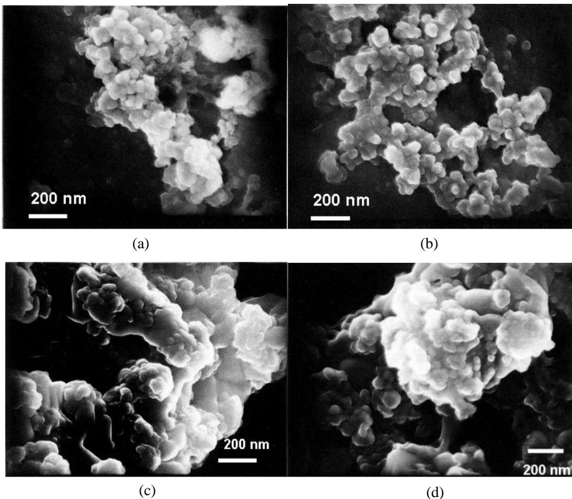
Figure 10. Image of PMMA synthesized with 10% (v/v) MMA and 0.5% (a), 1.5% (b) (w/v) SLS, 0.5% (c), 1.5% (d) CTAB (Parra et al., 2005)
