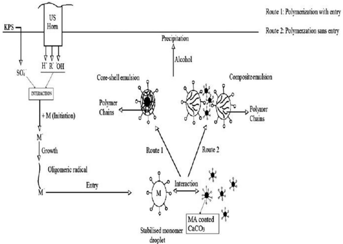
Figure 12. Mechanism of ultrasound initiated polymerization of PMMA/CaCO<sub>3</sub>
