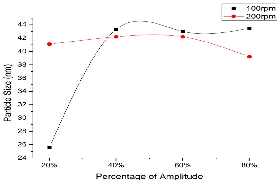
Figure 15. Change of Particle Size with Percentage of Amplitude and Agitation Speed
