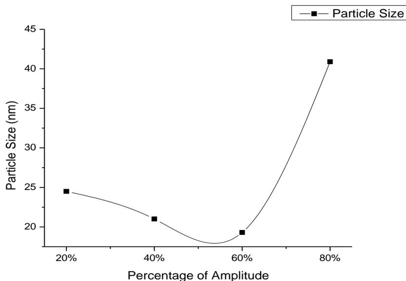
Figure 17. Change of Particle Size with Percentage of Amplitude with Probe Ultrasound of Pre-mixing Separation Method
