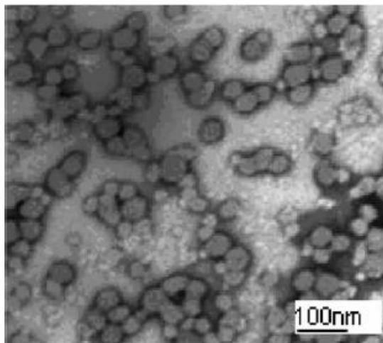
Figure 4. TEM pictures of nanosized poly-(styrene- $C_{12}N^+$ ) particles obtained by ultrasound irradiated emulsion polymerization (Zheng et al., 2007)
