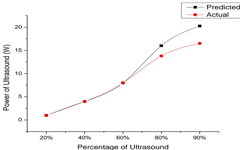
Figure 13. Power of Ultrasound with the Percentage of Amplitude of the Ultrasound Wave
