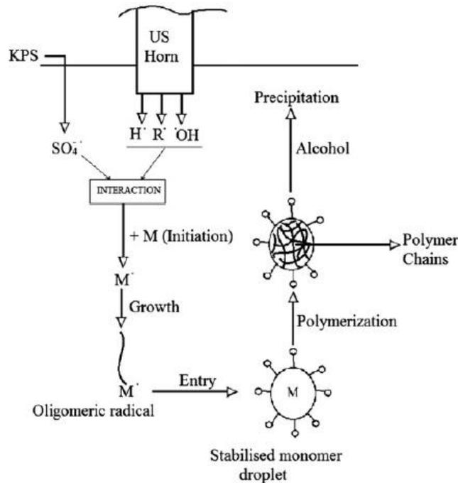
Figure 11. Mechanism of ultrasound initiated polymerization of MMA (Prasad et al., 2013)
