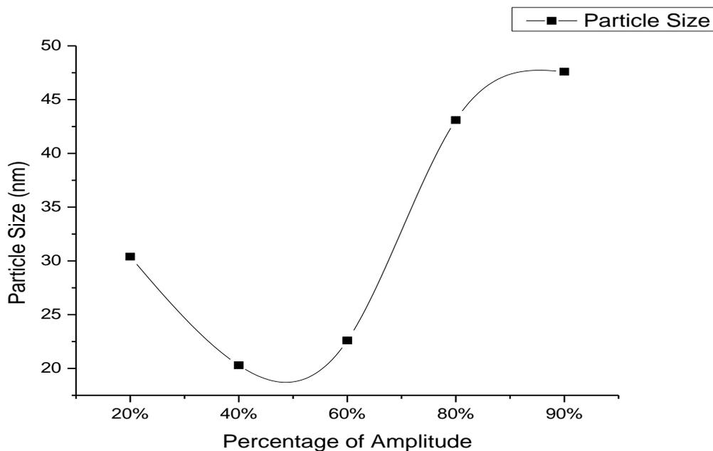
Figure 14. Change of Particle Size with Intensity of Ultrasound
