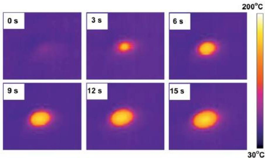
Figure 8. Temperature changes of a copolymer sample under HIFU within 15 seconds, recorded by infrared camera (Li et al., 2014)
