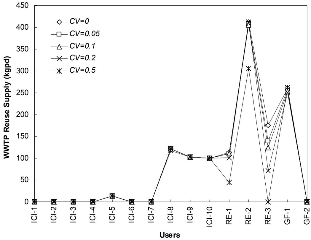
Figure 5.13 WWTP reuse supply with different coefficients of variation of demand
