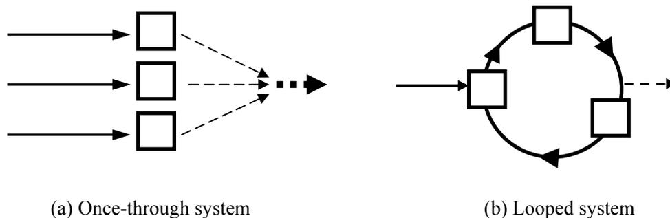
**Figure 1.1 Once-through and looped system**
