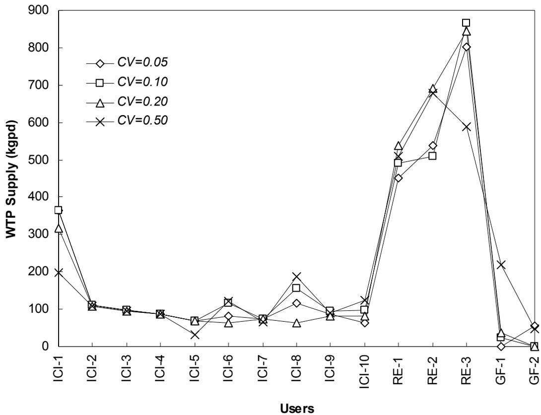
**Figure 5.18 WTP water supplies under different levels of quality variability using the quality chance-constraint of 96%**
