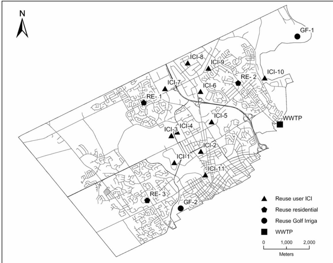
**Figure 5.3 Water reuse elements in the system, one WWTP, 15 major users**
