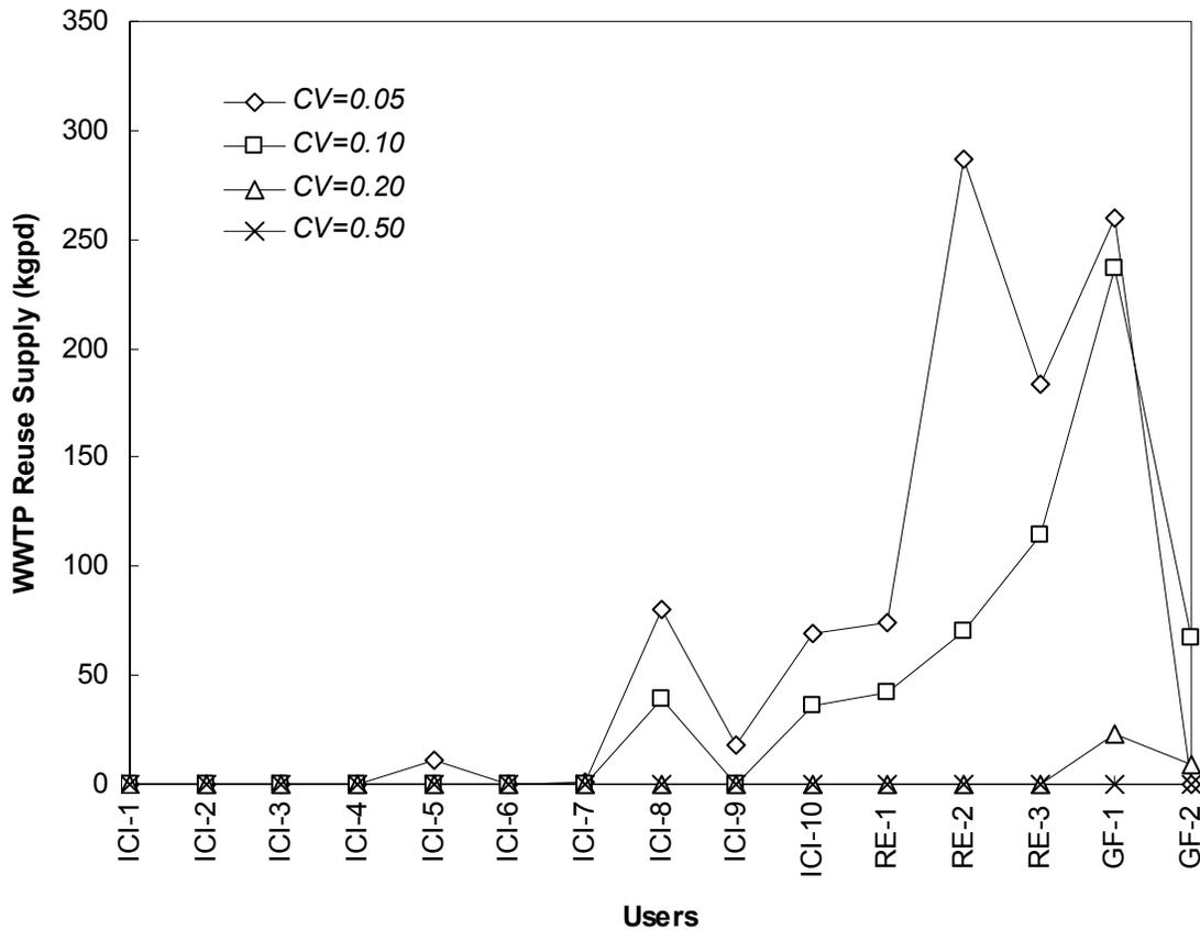
**Figure 5.19 WWTP reuse water supplies under different levels of quality variability using the quality chance-constraint of 96%**
