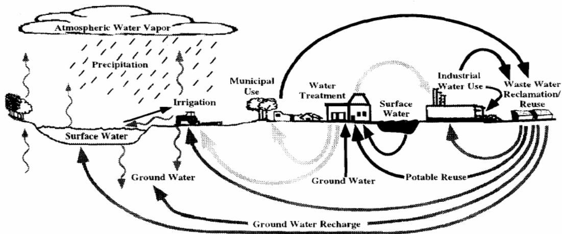
Figure 2.1 The concept of engineered urban water cycle with reuse (Asano *et al.*, 1996)
