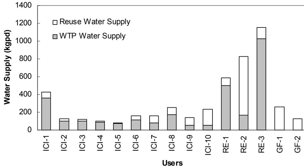
**Figure 5.7 WTP supply and total reuse water supply**
