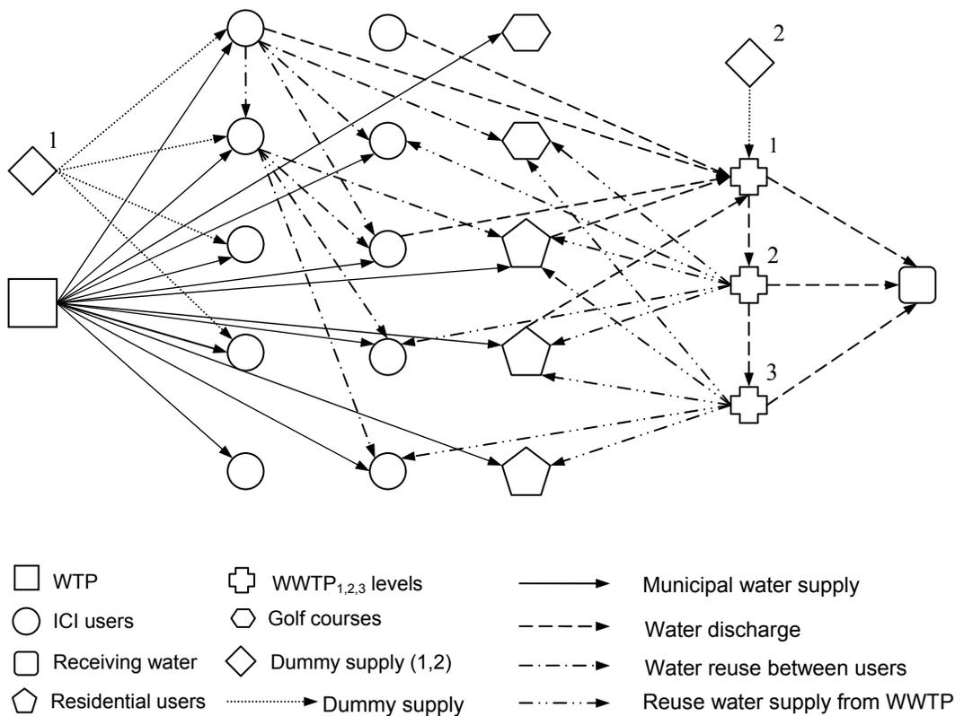
**Figure 5.4 Network diagram of the case study system**
