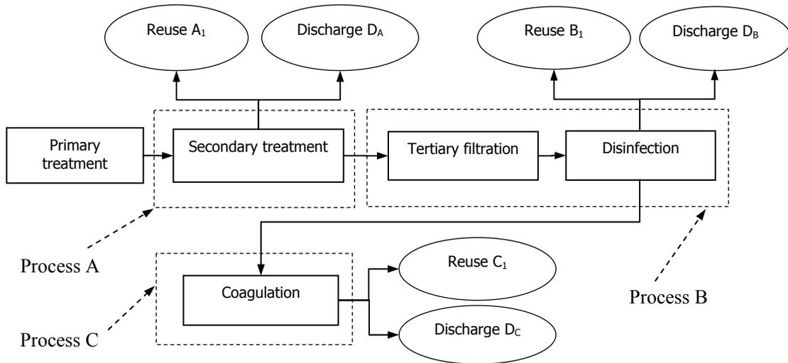
**Figure 4.1** An example of wastewater treatment train with 3 levels of processes
