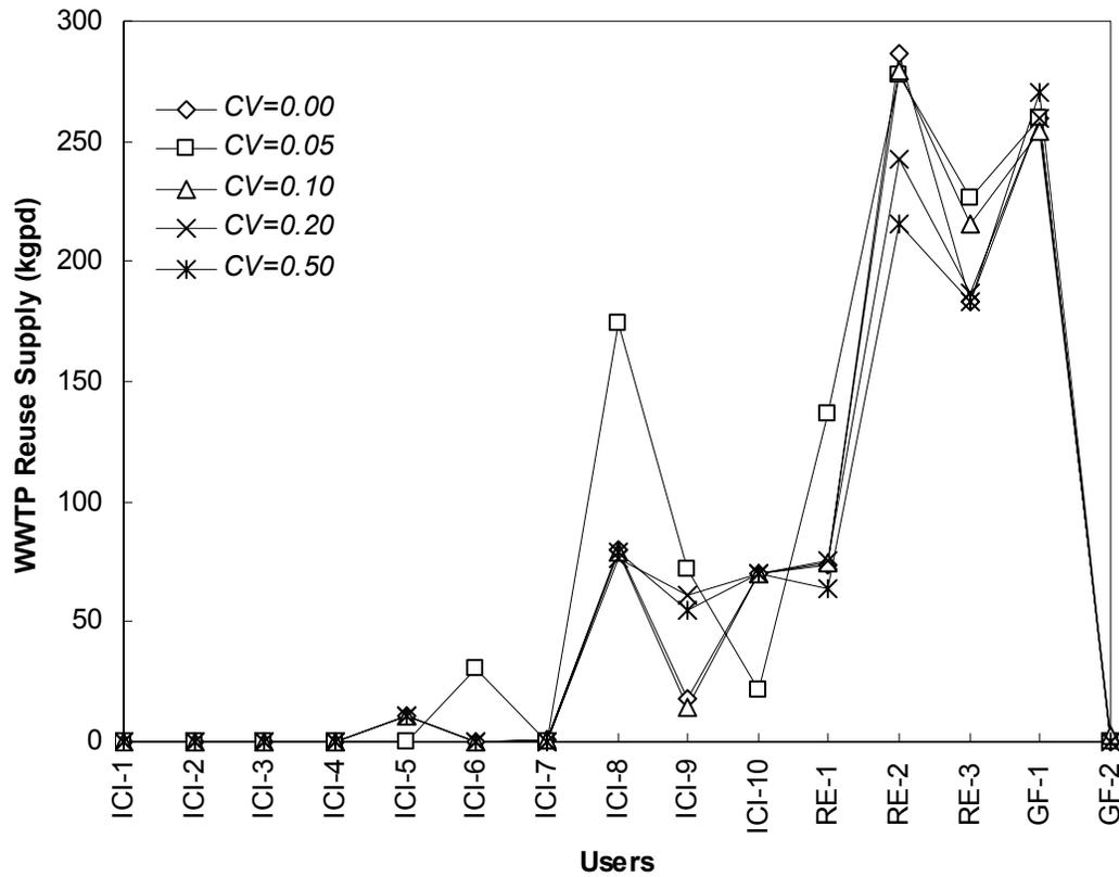
**Figure 5.24 WWTP reuse water supplies under 96% of quality chance-constraint with different levels of demand variability (coefficient of variation  $CV$ )**
