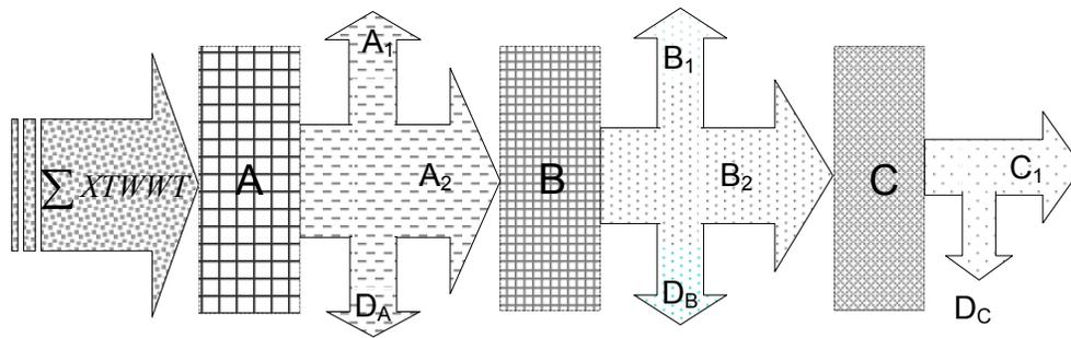
**Figure 4.2** Wastewater treatment train with 3 levels of processes ( $A, B, C$ )
