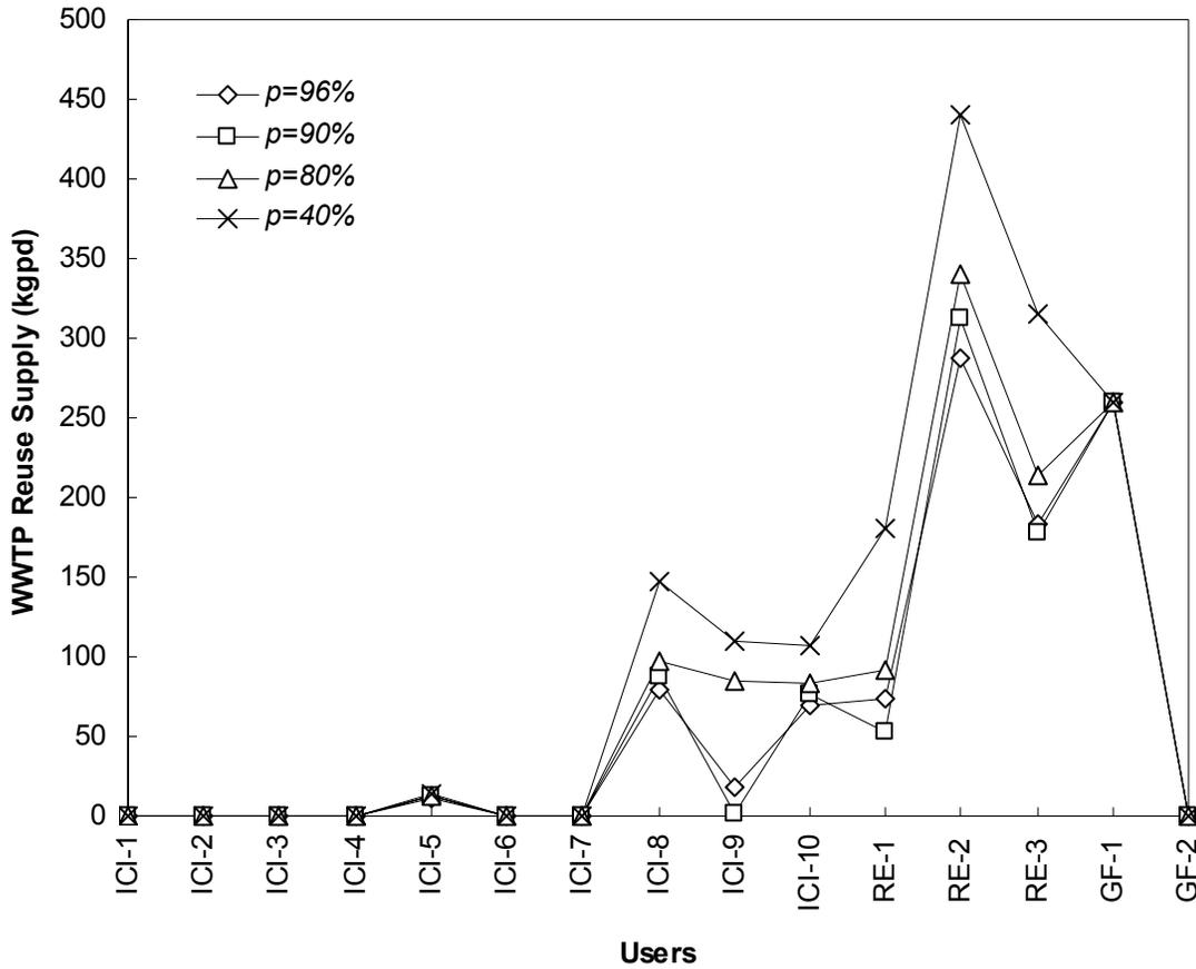
**Figure 5.17 WWTP reuse water supplies under different chance-constraints with quality variability  $CV=0.05$**
