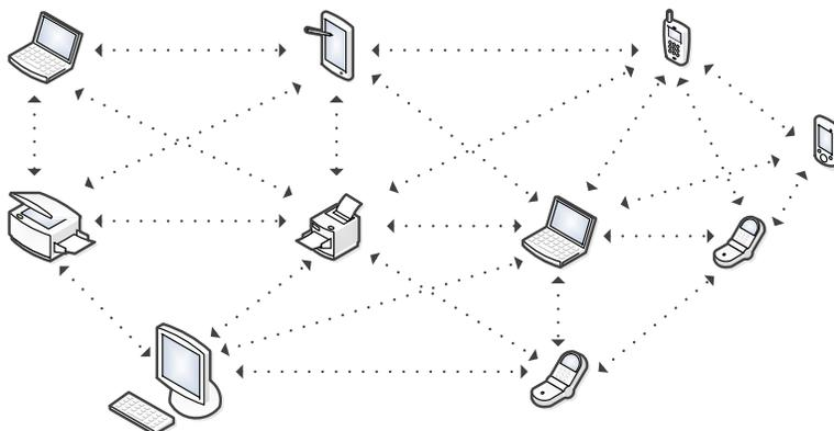
Figure 1.1: An illustration of wireless ad hoc network architecture.
