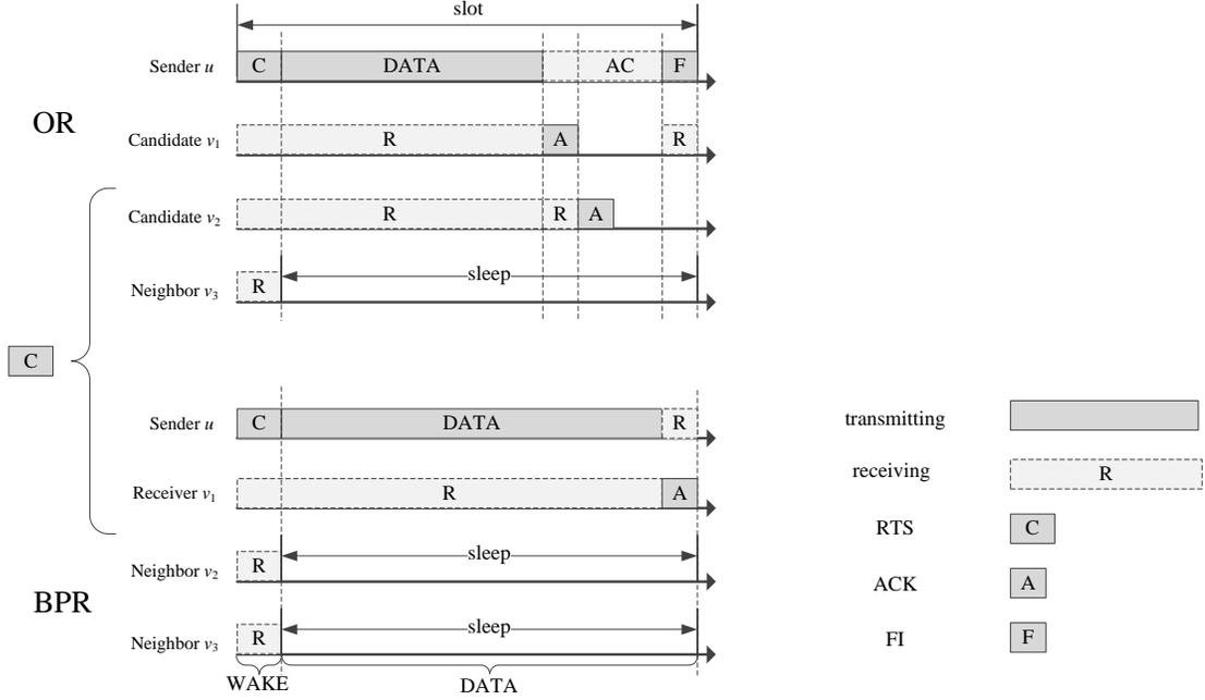
Figure 4.1: A timing diagram illustrating the routing operation within a single time slot.
