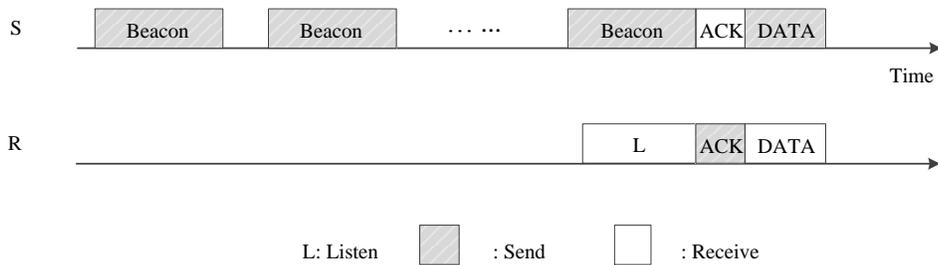
Figure 2.1: Illustration of the wake-up mechanism for communication under random sleep scheduling.
