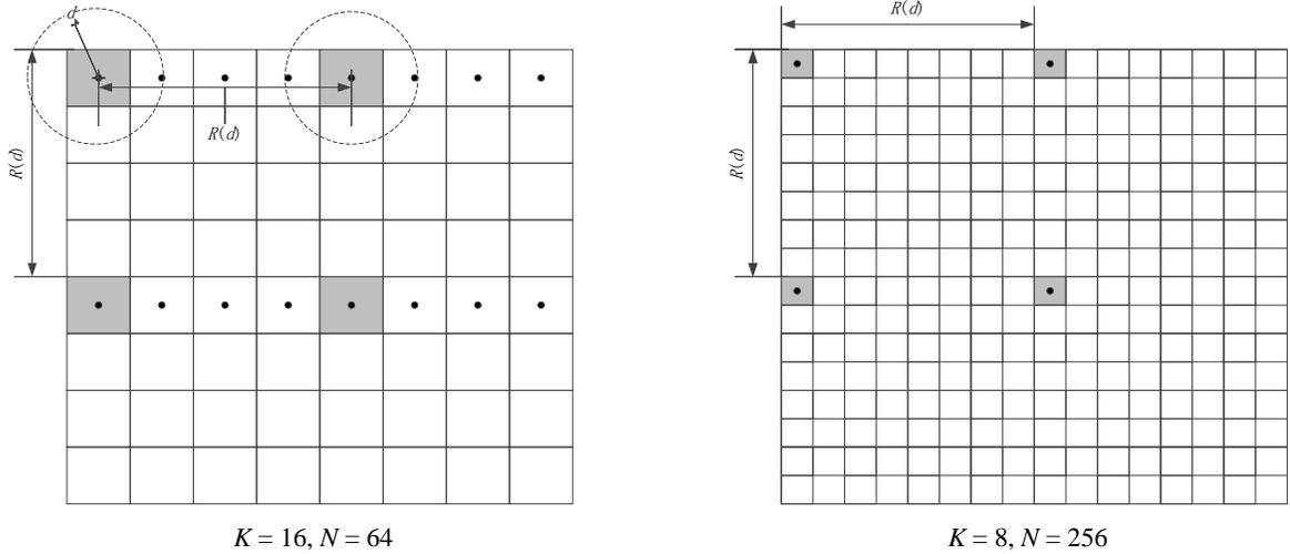
Figure 3.1: An illustration of restricted TDMA MAC under different node density scenarios with  $K = 16$  and  $K = 64$ , respectively. The dots at the center of each cell are the nodes, and grey cells can transmit simultaneously.
