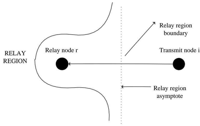
Figure 2.3: Relay region of transmit-relay node pair.
