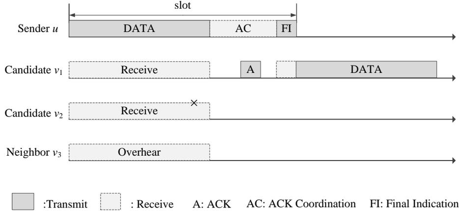
Figure 2.5: A timing diagram illustrating the OR operation within a single timeslot.
