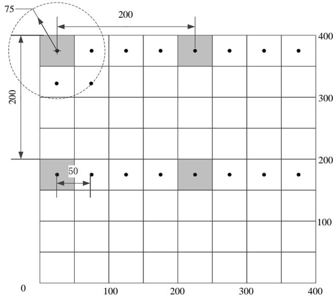
Figure 5.3: The topology for the example 1 and 2 with 64 nodes and 4 macro cells.
