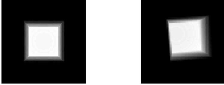
Figure 3.6: The initial guess of the DRR (left) and simulated target image using the transformation parameter set  $\mathbf{s}$  as  $(5^\circ, 5^\circ, 5^\circ, 0.1, 0.1, 0.1)^T$  (right).
