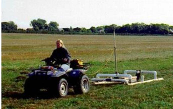
**Figure 2.3: Soil conductivity measurements with the EM-38 on an all-terrain vehicle**
