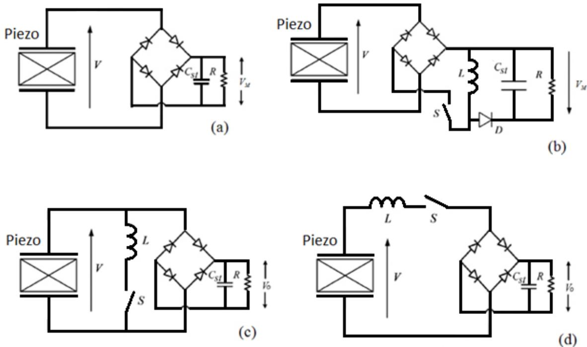
FIGURE 1-3: STANDARD HARVESTING CIRCUIT AND THREE NONLINEAR MODIFICATIONS. A) STANDARD MODEL. B) SWITCH PRECHARGED INDUCTOR. C) PARALLEL SSHI. D) SERIES SSHI. [9]
