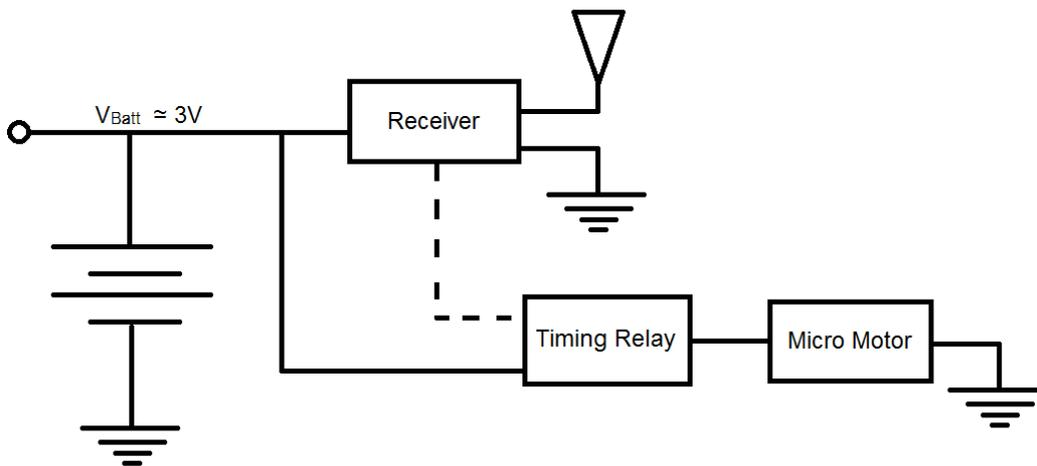
FIGURE 4-2: LOAD CIRCUITRY OPERATING AT 3 VOLT LOGIC
