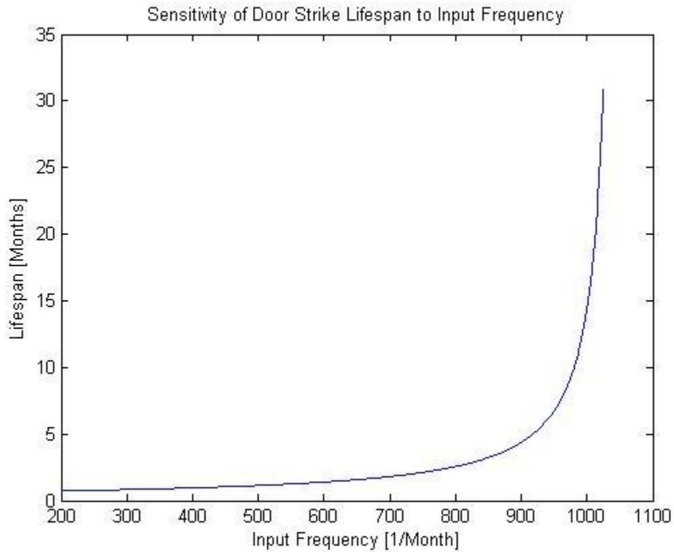
FIGURE 3-7: SENSITIVITY OF DOOR STRIKE LIFESPAN TO INPUT FREQUENCY
