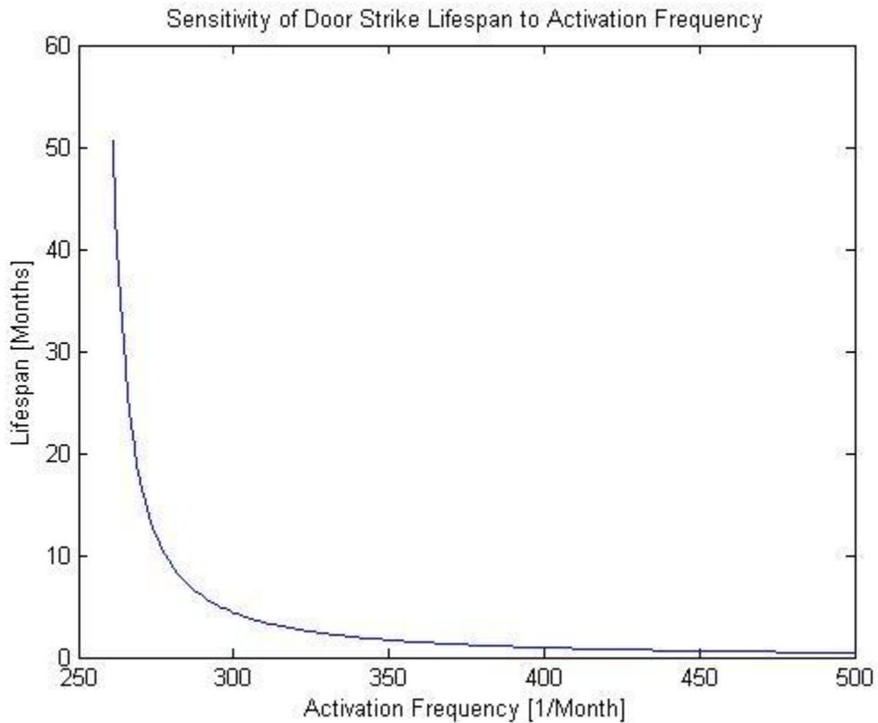
FIGURE 3-8: SENSITIVITY OF DOOR STRIKE LIFESPAN TO ACTIVATION FREQUENCY
