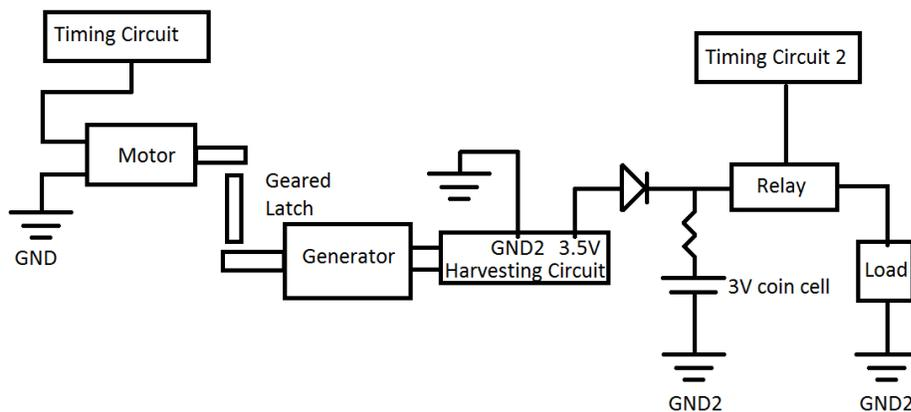
FIGURE 4-3: HYBRID DOOR STRIKE EXPERIMENTAL DIAGRAM
