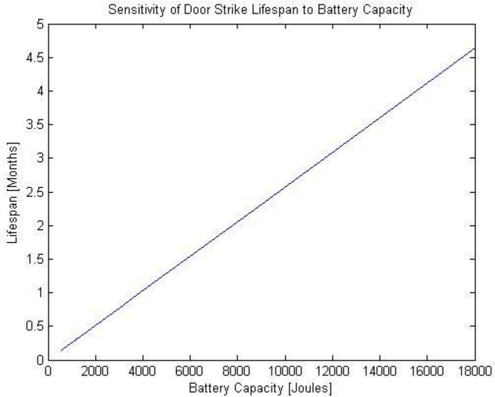
FIGURE 3-4: SENSITIVITY OF DOOR STRIKE LIFESPAN TO BATTERY CAPACITY
