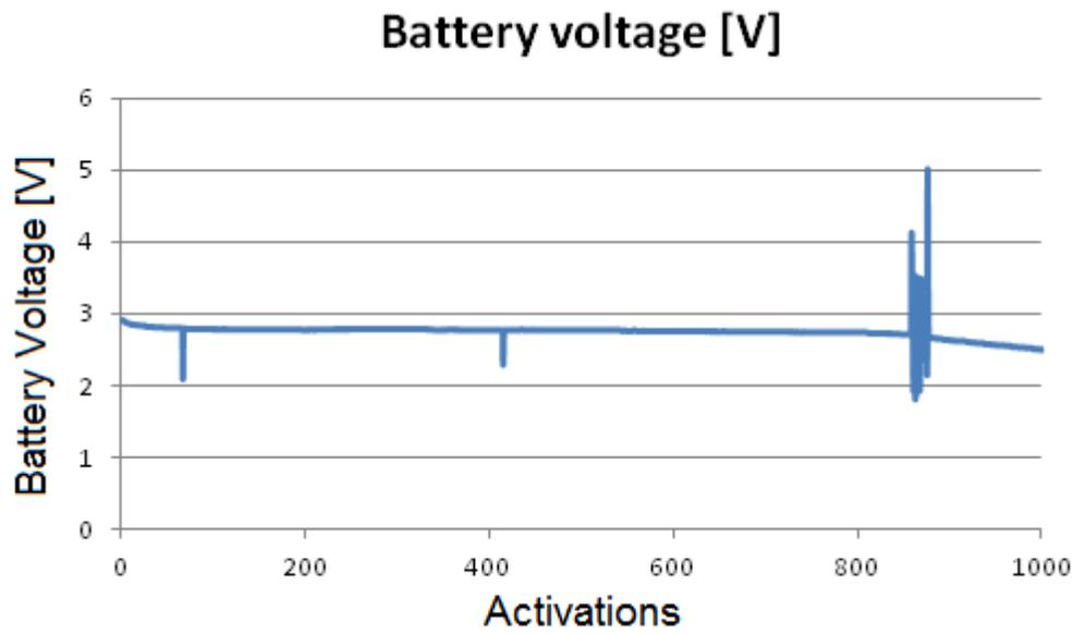
FIGURE 4-5: BATTERY VOLTAGE DROP FOR AN A/I RATIO OF INFINITY (NO HARVESTING)
