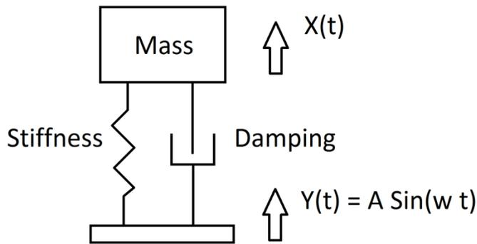
FIGURE 1-1: SINGLE DEGREE OF FREEDOM BASE EXCITATION WITH SINUSOIDAL INPUT
