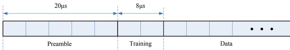
Figure 4.2: The OFDM packet structure for WARP implementation
