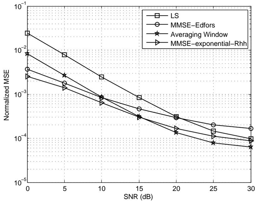
Figure 4.14: Normalized MSE for channel model D2
