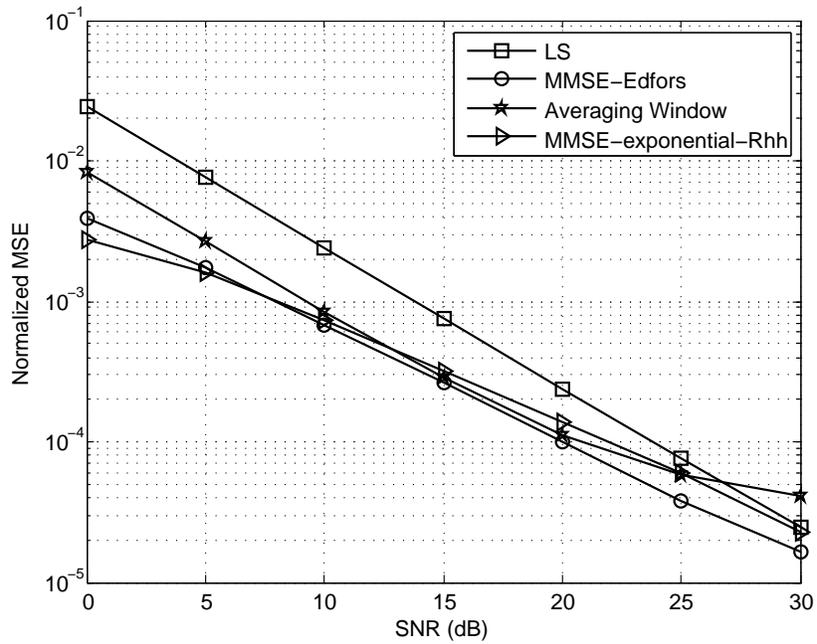
Figure 4.15: Normalized MSE for channel model E1
