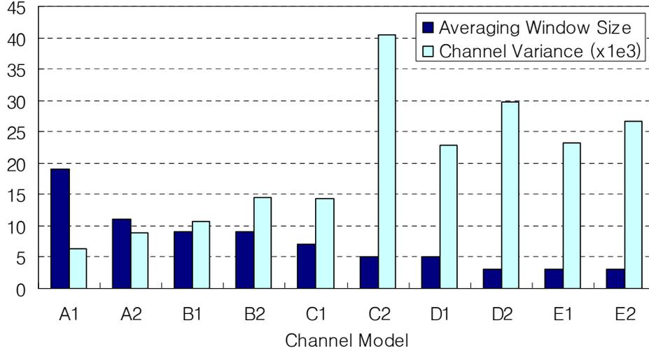
Figure 4.20: Relationship between the averaging window size and the frequency selectivity
