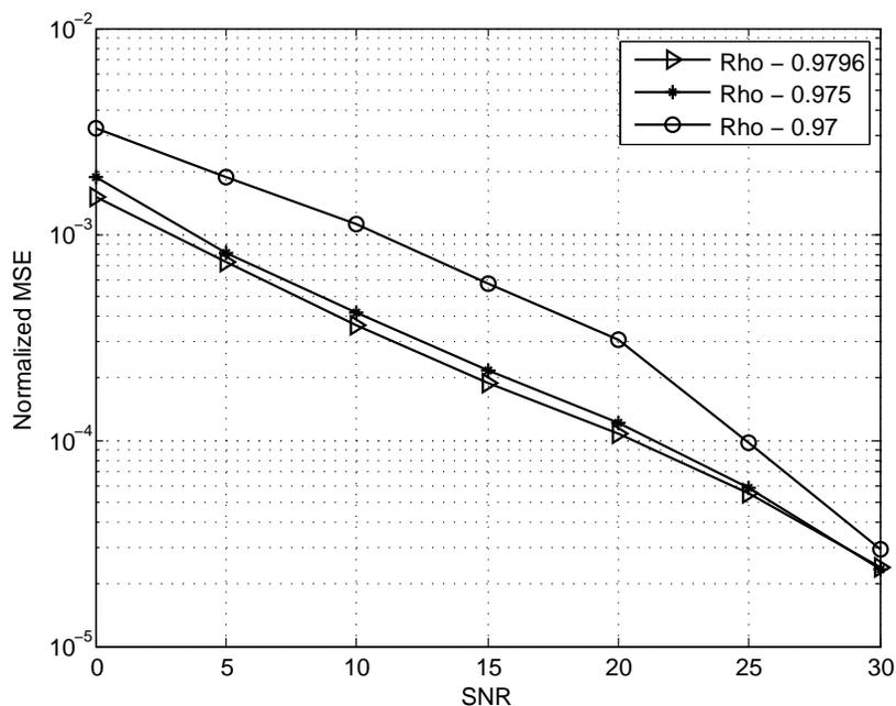
Figure 4.19: Influence of  $\rho$  in MMSE-exponential-Rhh estimator for channel model A1
