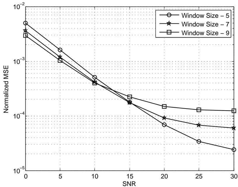
Figure 4.17: Effects of averaging window size for channel model C1
