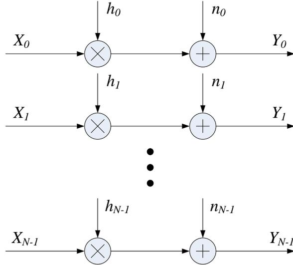
Figure 2.2: The OFDM system, modeled as parallel Gaussian channels
