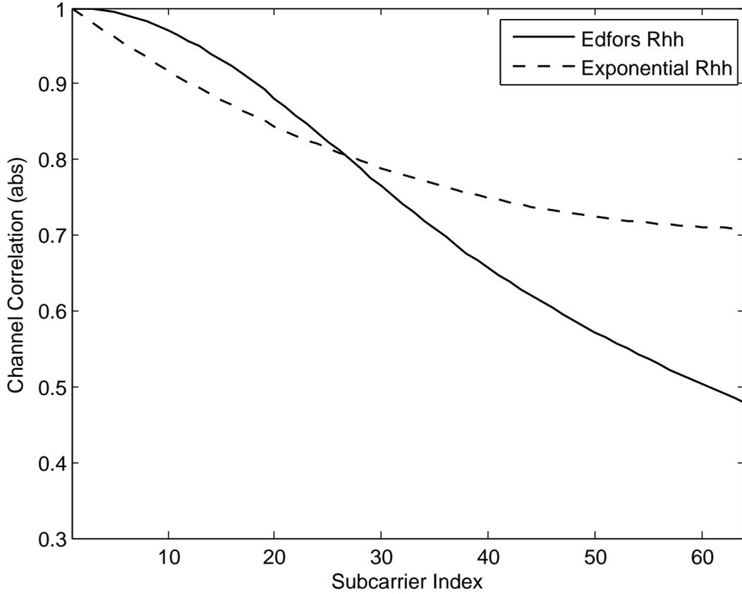
Figure 3.2: The channel correlation of the attenuation at  $m = 1$  with the rest of attenuations in case where  $N = 64$ ,  $\tau_{rms} = 15ns$ ,  $\tau_{max} = 80ns$ , and  $\rho = 0.98$
