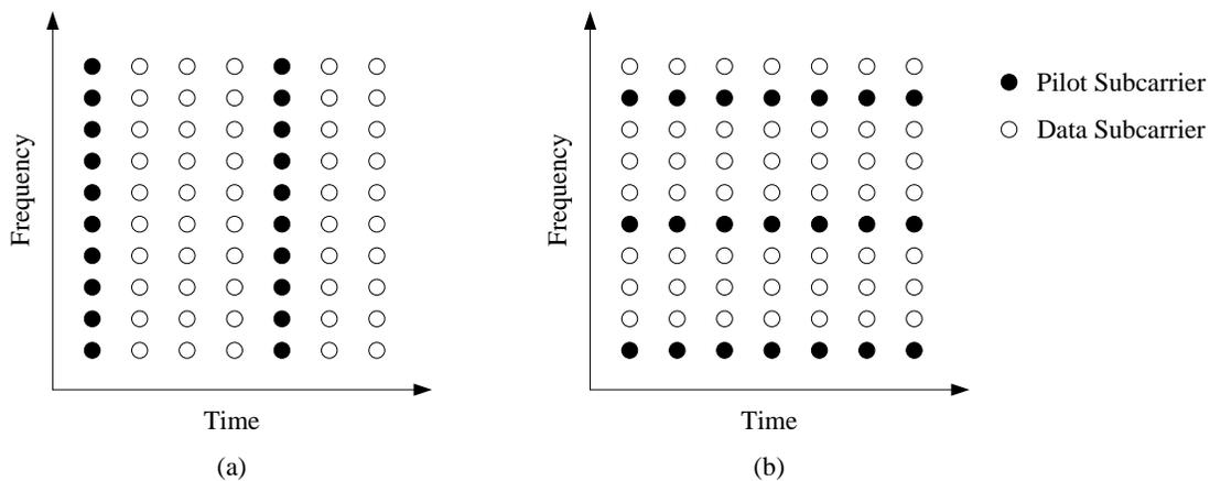
Figure 3.1: Two different types of pilot arrangement: (a) block-type pilot arrangement and (b) comb-type pilot arrangement
