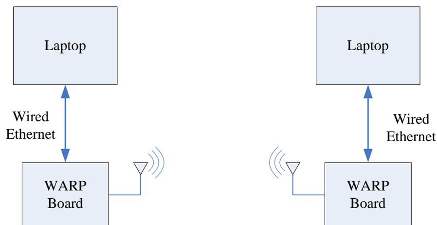
Figure 4.3: The equipment setup for channel measurement
