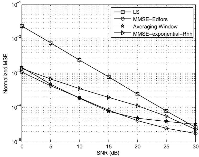
Figure 4.7: Normalized MSE for channel model A1
