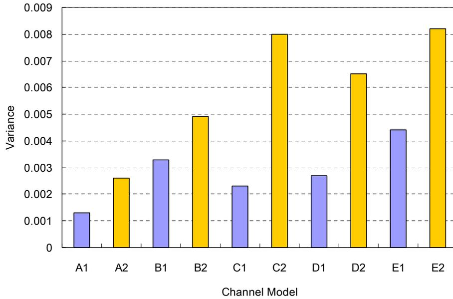
Figure 4.6: Variance of channel frequency response over time
