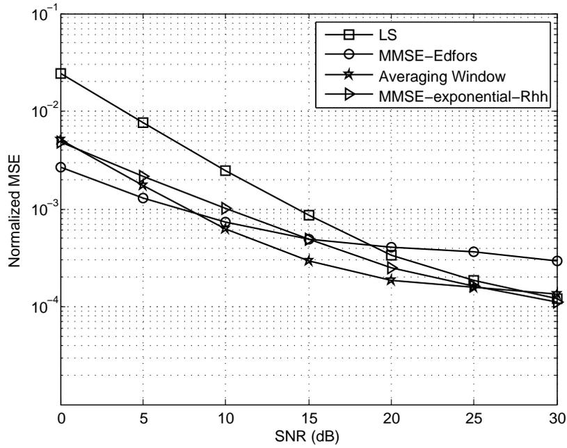
Figure 4.12: Normalized MSE for channel model C2
