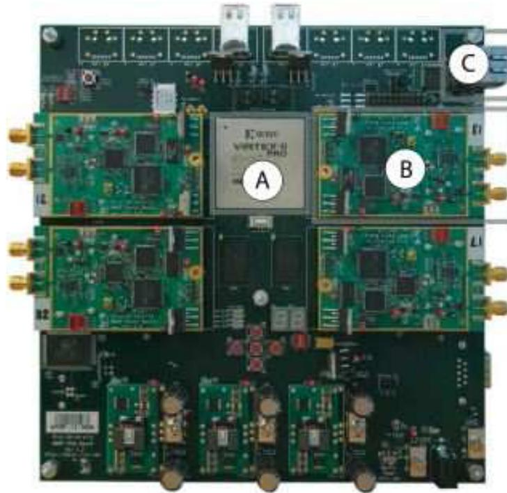
Figure 4.1: The WARP board as the IEEE 802.11 interface
