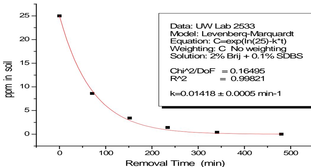
**Figure 16. Removal Time using 2% Brij + 0.1% SDBS solution.**
