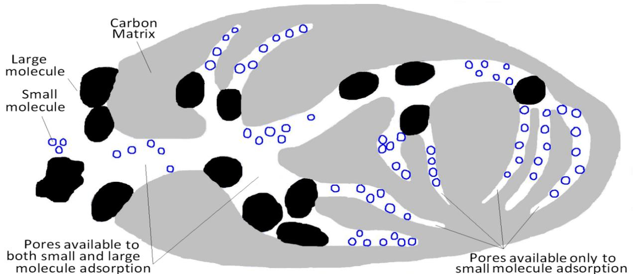
**Figure 6. Molecular screening in the micropores of an activated carbon filter.**
