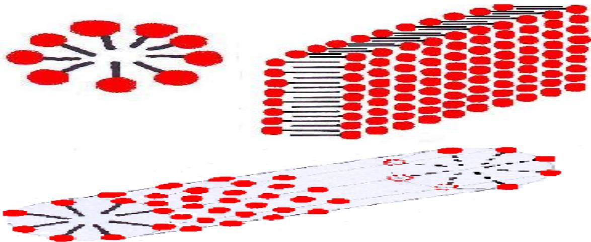
Figure 4. Schematic diagram of micelles. [http://barrett-group.mcgill.ca/teaching/liquid\\_crystal/LC05.htm](http://barrett-group.mcgill.ca/teaching/liquid_crystal/LC05.htm)
