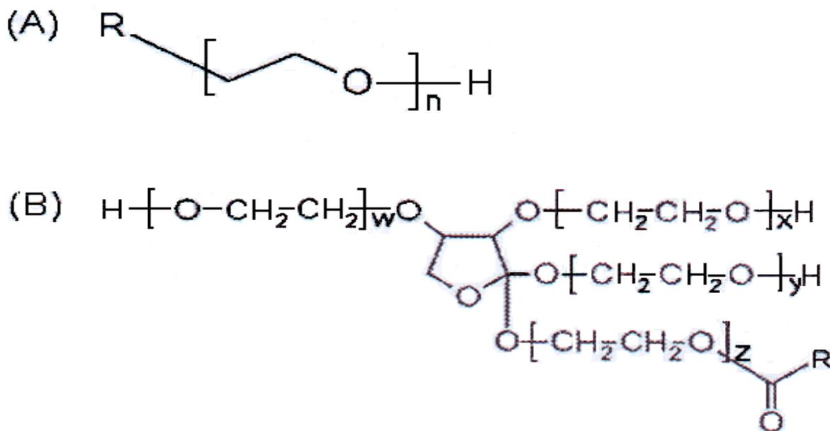
Figure 9. General formula: (A) Brij (polyethoxylates), (B) Tween (sorbitan derivatives). R = alkyl chain, and n = number of ethoxylate groups present in the molecule. (Franzetti et. al, 2008)
