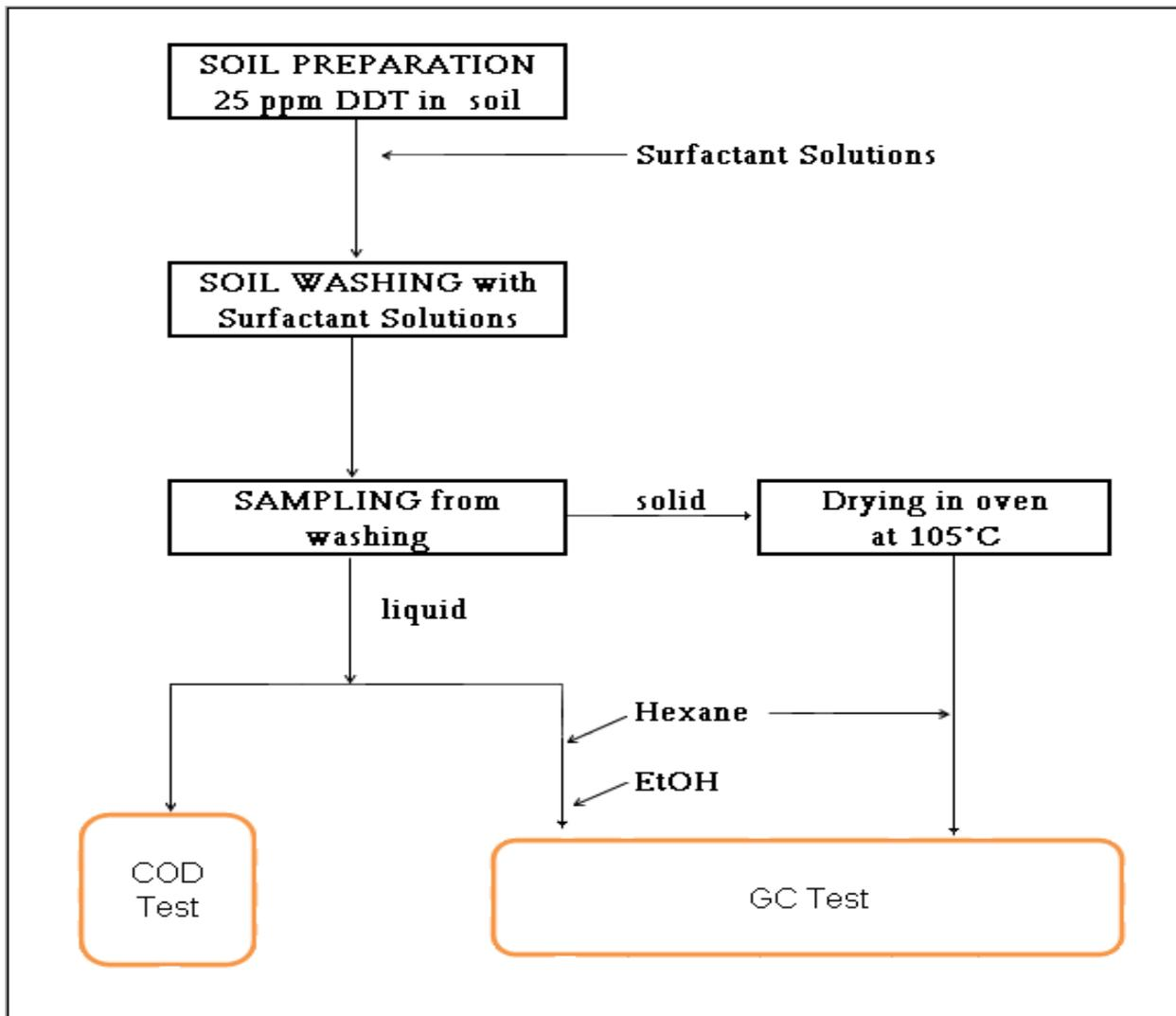
Figure 8. Flow sheet of the soil washing process used in this work. COD: Chemical oxygen demand, GC: Gas Chromatographic.
