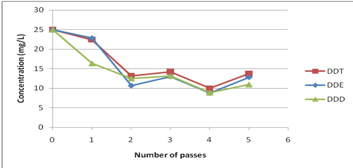
**Figure 17: Change in contaminant concentration in the effluent from an activated carbon adsorption column (5 g), using 1% Brij 35 + 0.1% SDBS aqueous solution, 25 mL per pass.**
