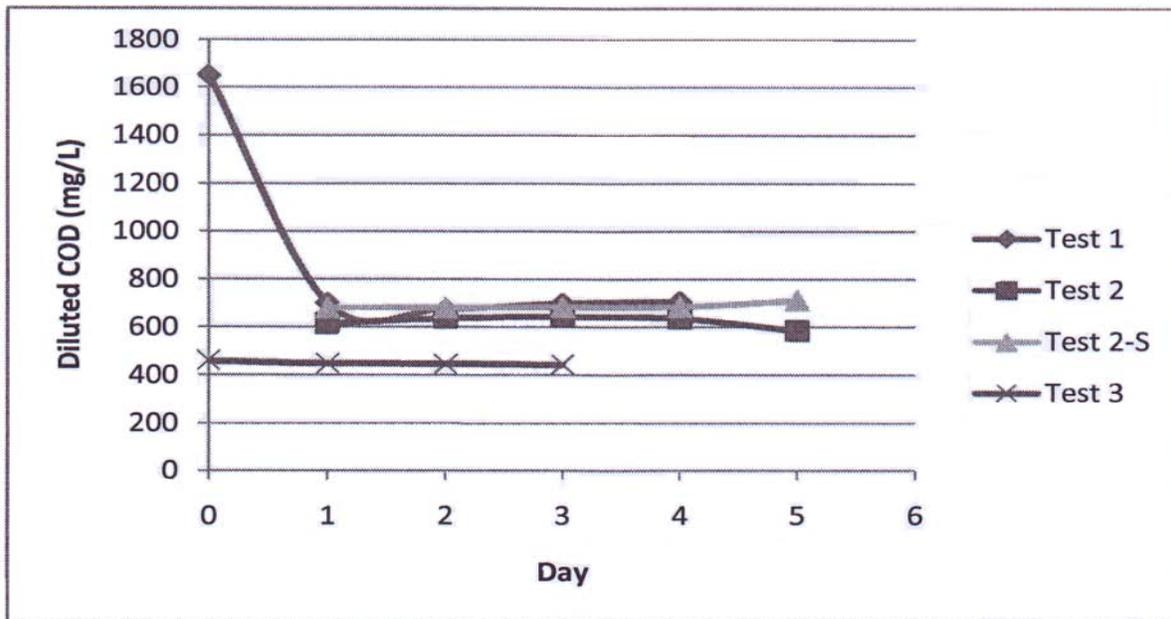
Figure 12. Surfactant biodegradation test. Test-1 and Test 2: 1% Tween 80 non-sterilized; Test 2-S: sterilized control; Test-3: mixture of 0.5% Tween 80 and 0.5% Brij 35 non-sterilized.
