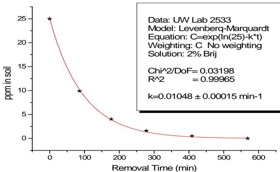
Figure 15. Removal Time using 2% Brij solution.
