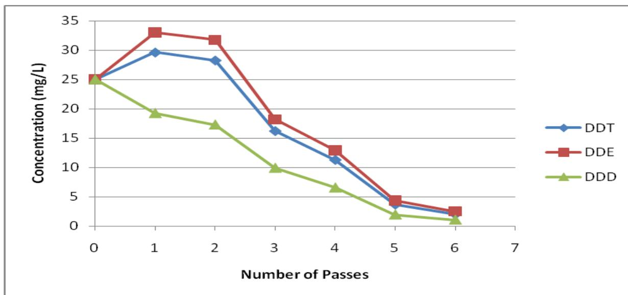
**Figure 18: Change in DDT-related contaminant concentration in a 1% Brij 35 + 0.1% SDBS solution passed through 4 g beds of activated carbon, replaced after each pass.**
