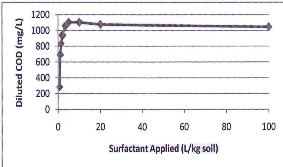
Figure 11. Second adsorption test: fixed amount of surfactant with varying amount of soil.
