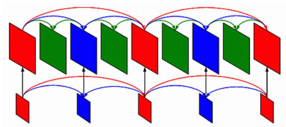
Figure 2.5: Multi-layer structure with additional inter-layer prediction (black-arrows) [4]
