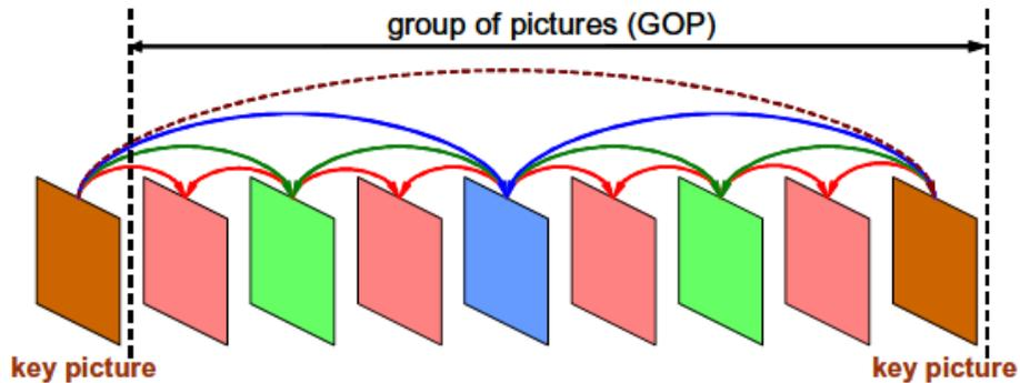
Figure 2.6: Hierarchical prediction structure with 4 dyadic levels [22]
