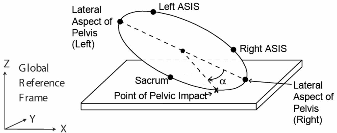
**Figure 3-4 Definition of hip proximity angle.** The hip proximity angle, which is shown by alpha in the diagram, is an absolute angle that reflects how near the site of pelvic impact is to the lateral aspect of the hip. An angle of 0 degrees indicates direct impact to the lateral aspect to the hip, while +90 degrees reflects impact to the anterior aspect of the pelvis and -90 degrees indicates impact to the posterior aspect of the pelvis.
