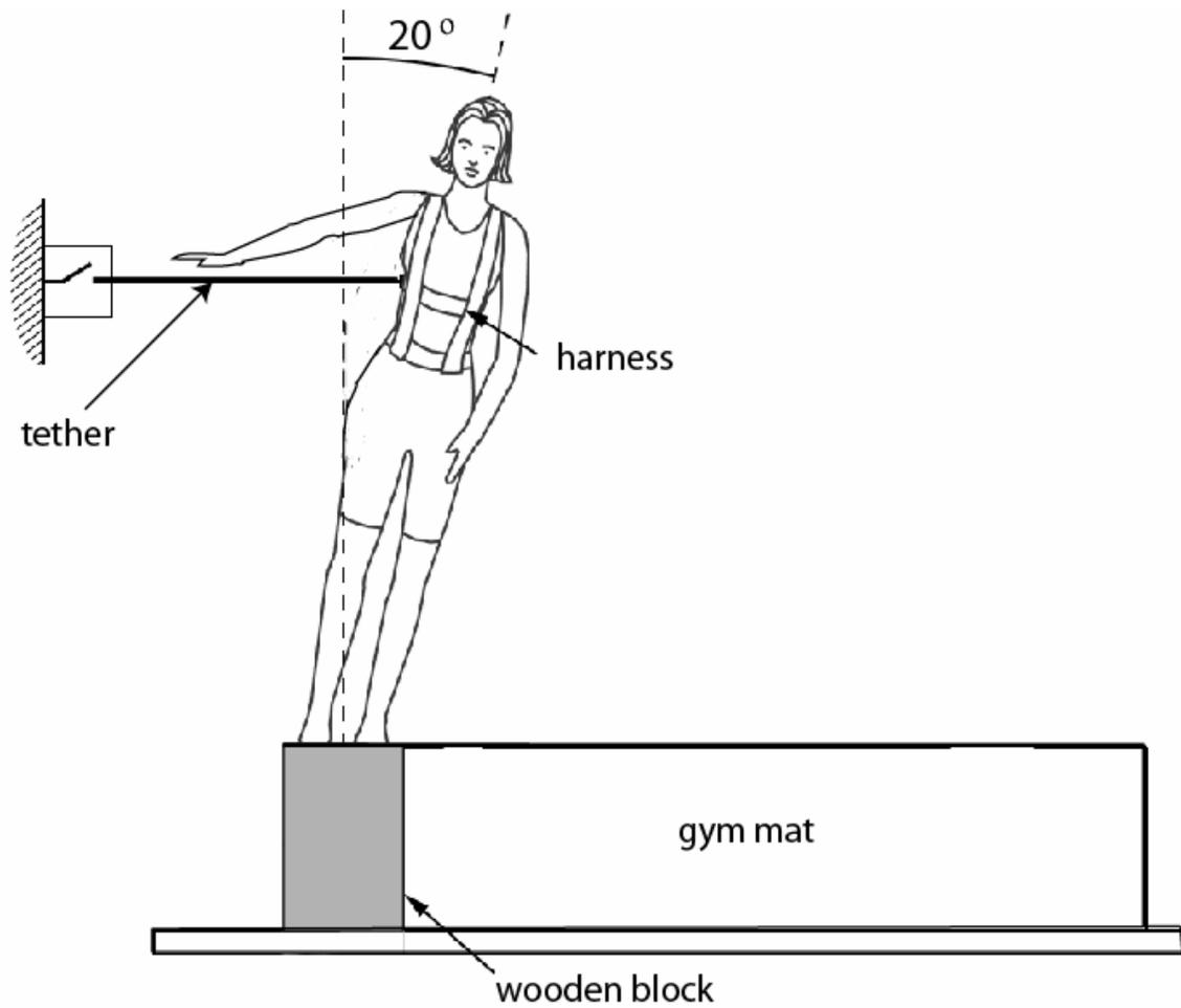
Figure 3-1 Experimental setup. A sideways fall was unexpectedly initiated by releasing a tether, which held the subject at a 20° lean angle.
