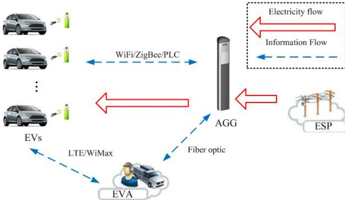
Figure 3.2: System Model in PMQC
