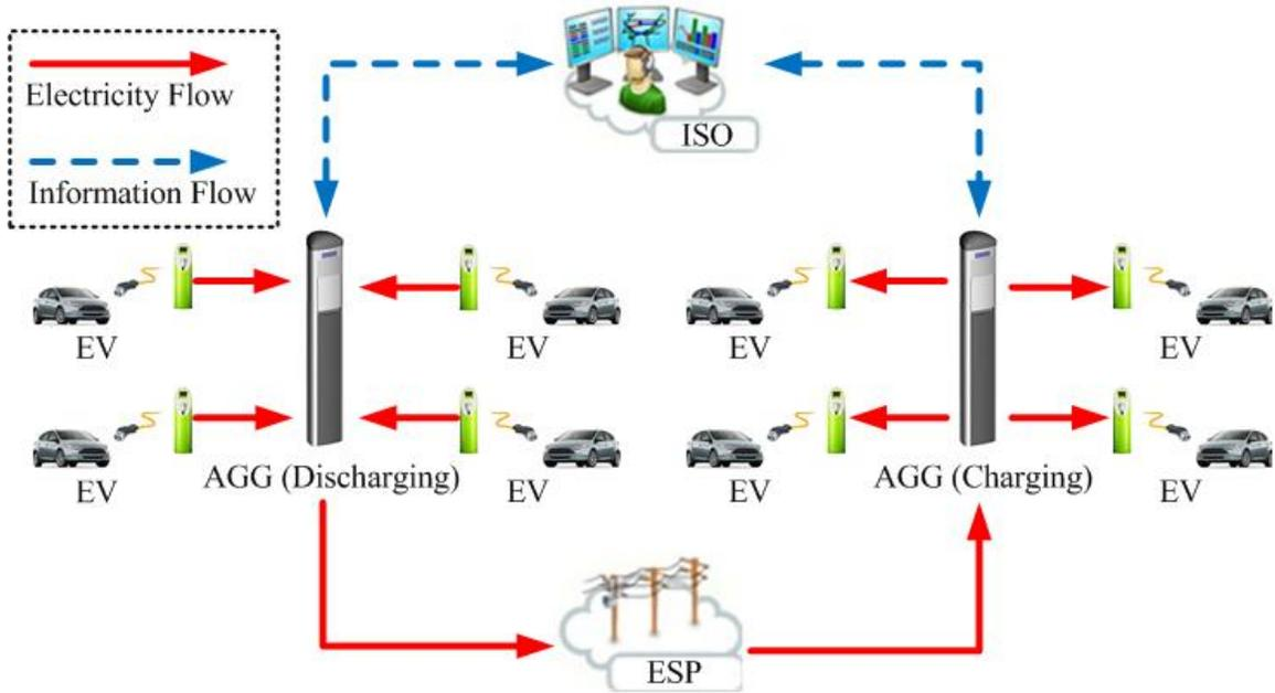
Figure 1.3: Structure of V2G Network
