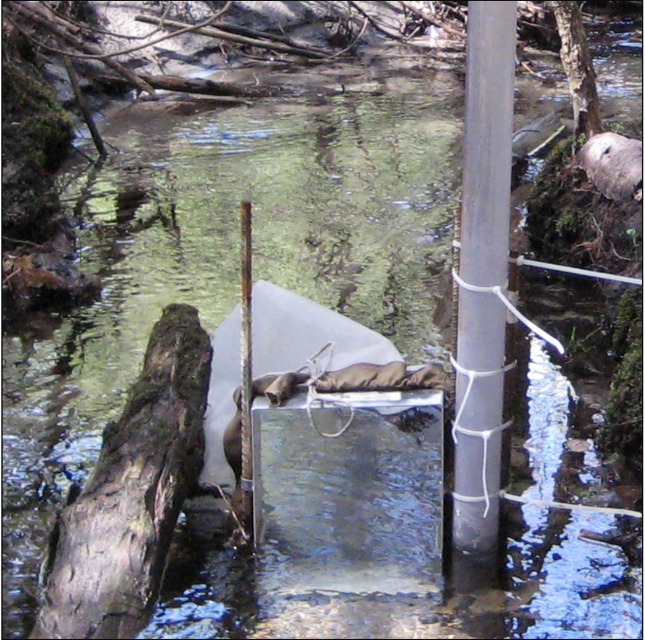
**Figure 2** Drift trap (20 cm by 30 cm by 7 cm) installation at KET 1 (site not used in this thesis because channel was permanent). Rebar post attached to each side of the aluminum drift trap secure it to the channel bed and support the 100 cm long, clear 2" PVC pipe used to record maximum water level.
