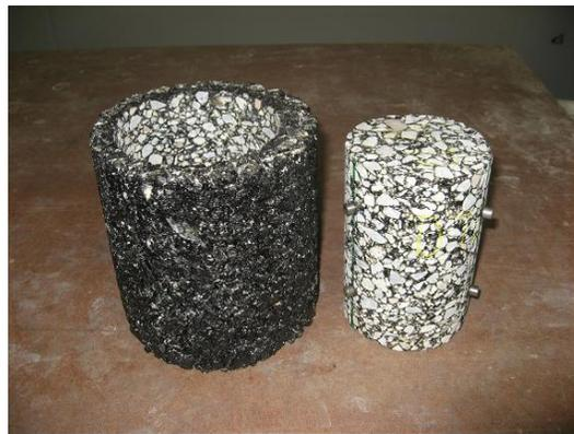
**Figure 5.3 Cored Samples for Dynamic Modulus Test**
