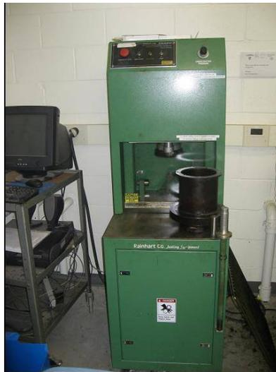
**Figure 5.1 Rainhart Superpave Gyratory Compactor**
