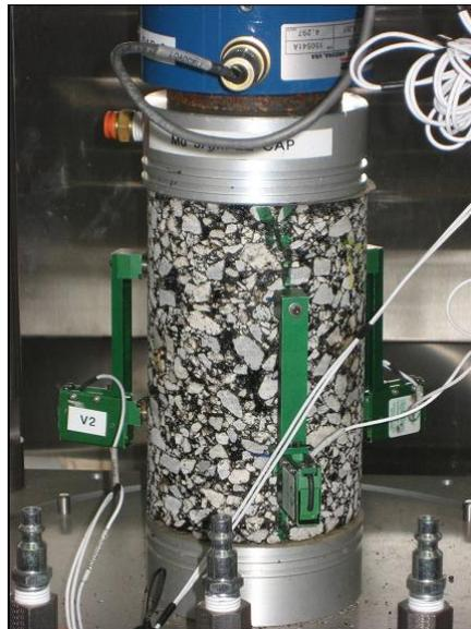
**Figure 5.5 Sensor Configuration for Dynamic Modulus Testing**
