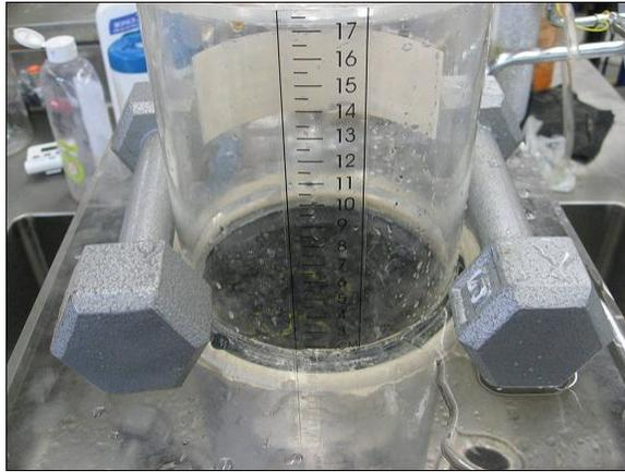
**Figure 5.7 Permeameter With Sample in Place**
