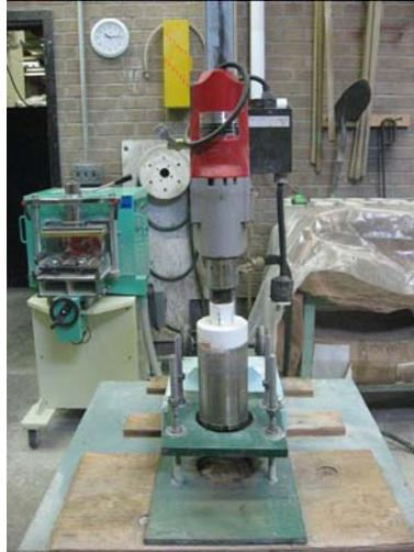
**Figure 5.2 Coring Apparatus**
