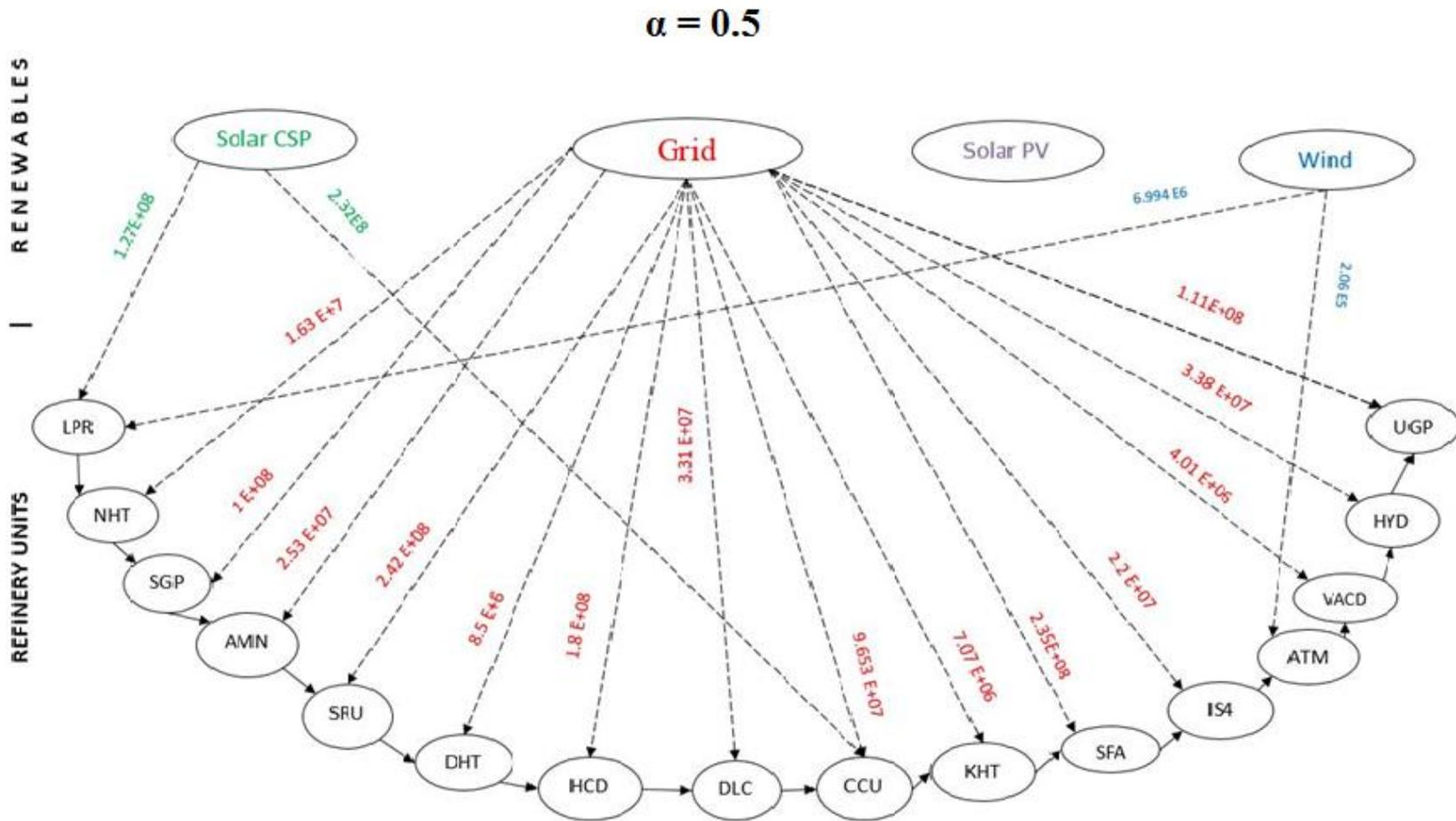
Figure 14. Superstructure for Energy Resources Distribution and Refinery Units at an  $\alpha$  value of 0.5
