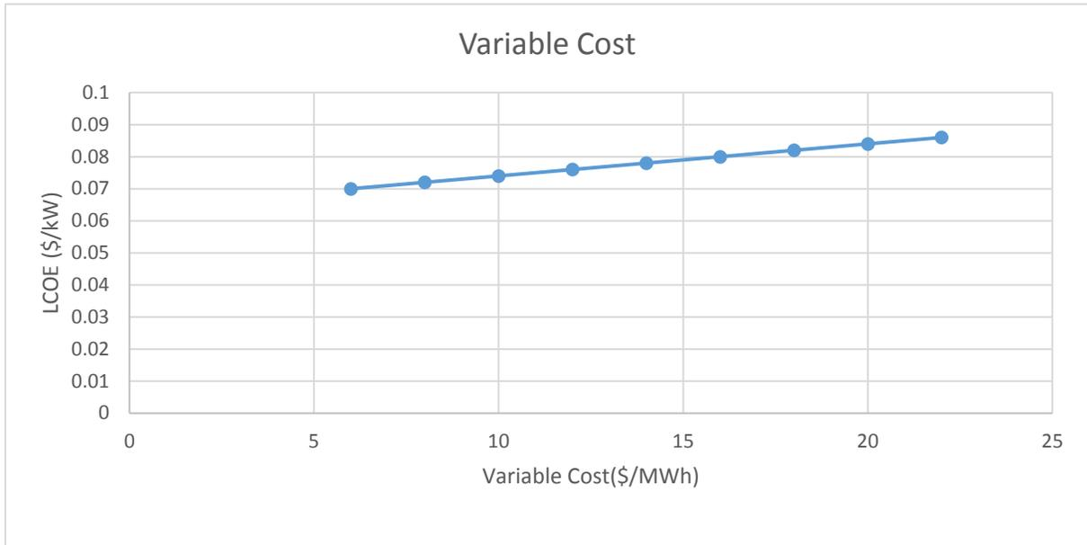
Figure 32. LCOE for Wind energy at different values of variable cost
