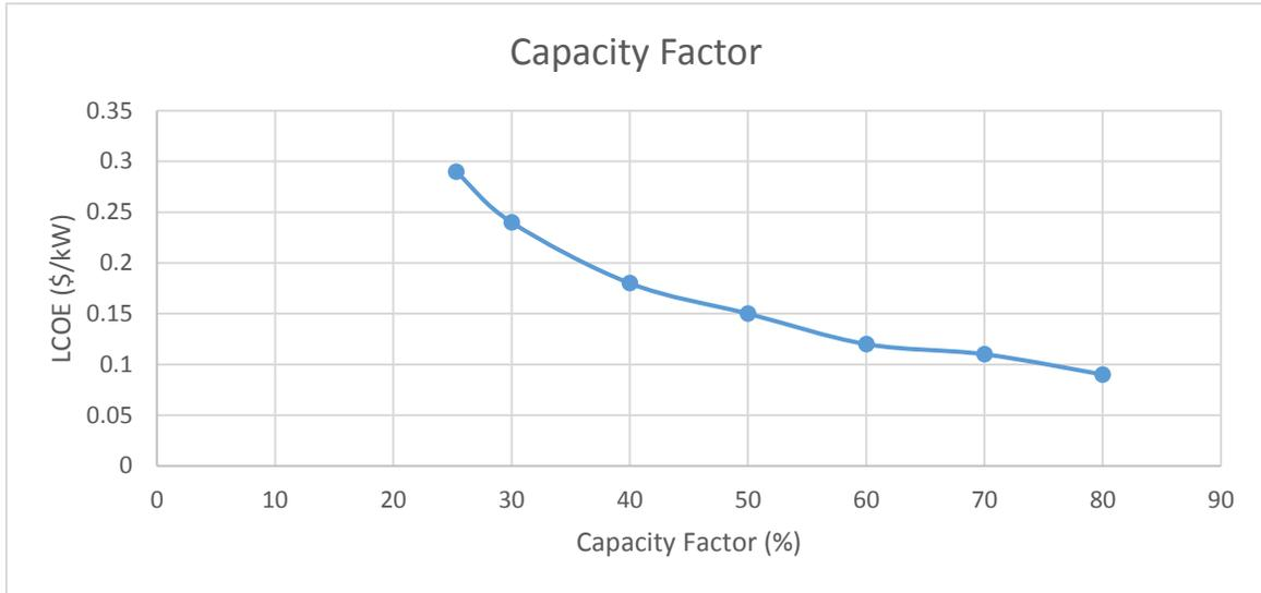
Figure 23. LCOE for Solar CSP with different capacity factor values
