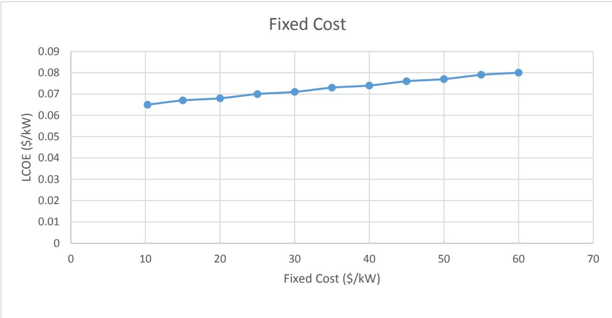
Figure 31. LCOE for Wind energy at different values of fixed cost
