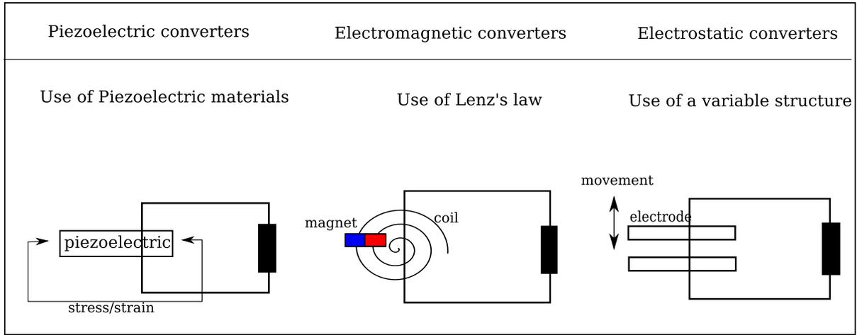
Figure 1.1: Mechanical-to-electrical converters [11]
