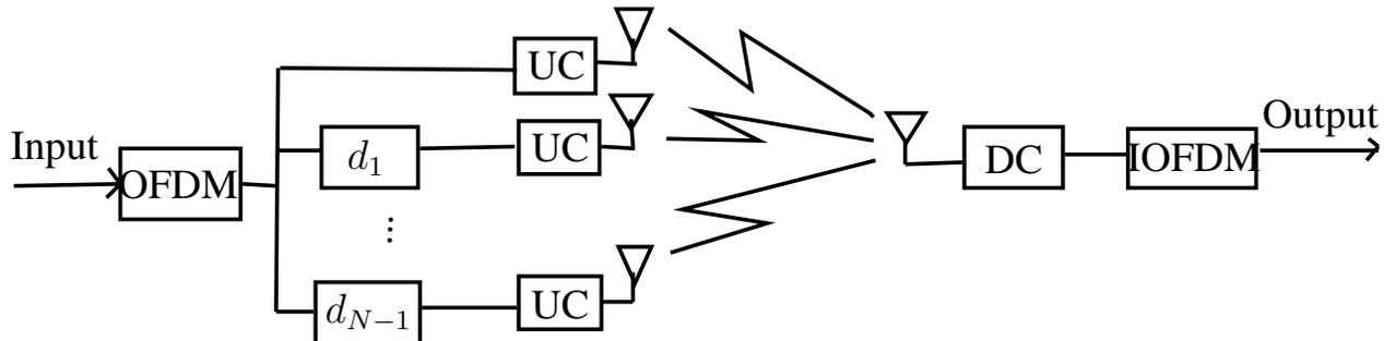
Figure 1.5: Phase Diversity Block Diagram
