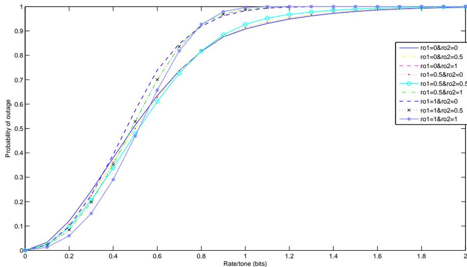
Figure 2.8: Two-user Gaussian interference channel with  $N=4$  and  $\text{SNR}=0\text{dB}$  (Frequency-flat)
