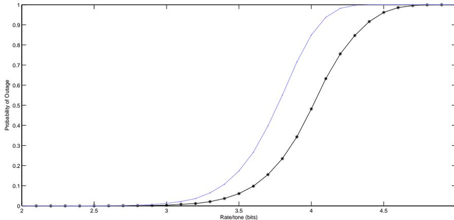
Figure 2.12: Two-user Gaussian interference with and without decoding interference option
