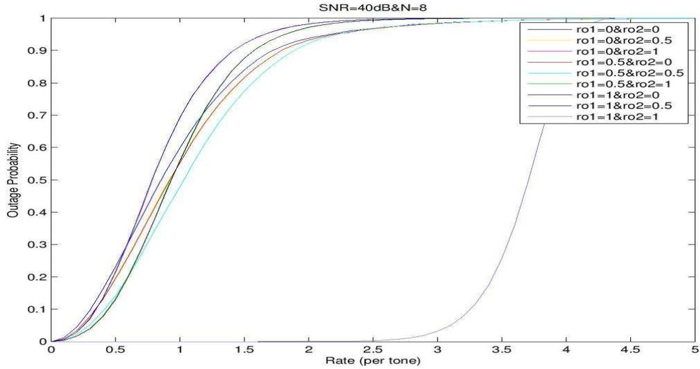
Figure 2.9: Two-user Gaussian interference channel with  $N=8$  and  $\text{SNR}=40\text{dB}$
