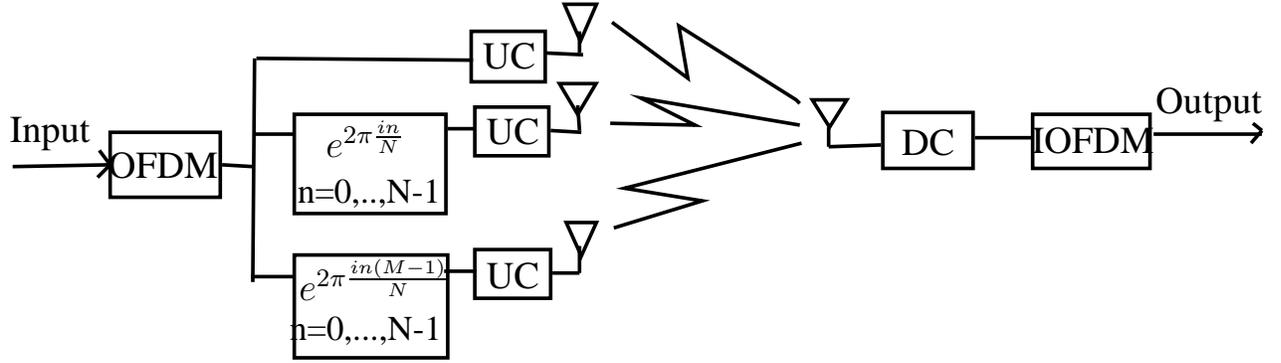
Figure 1.4: Subcarrier Diversity Block Diagram
