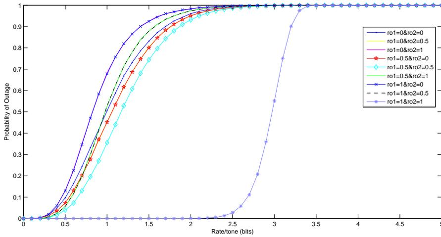
Figure 2.10: Two-user Gaussian interference channel with  $N=4$  and  $\text{SNR}=30\text{dB}$  (Frequency-selective)
