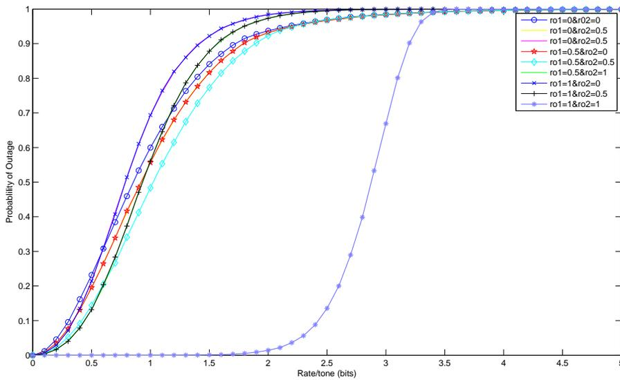
Figure 2.5: Two-user Gaussian interference channel with  $N=4$  and  $\text{SNR}=30\text{dB}$  (Frequency-flat)
