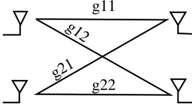
Figure 1.1: Two-user interference channel
