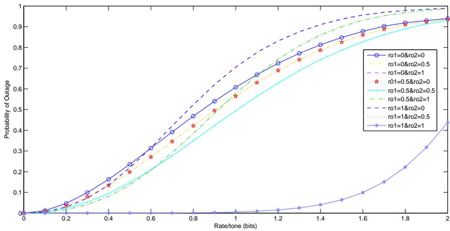
Figure 2.6: Two-user Gaussian interference channel with  $N=4$  and  $\text{SNR}=20\text{dB}$  (Frequency-flat)
