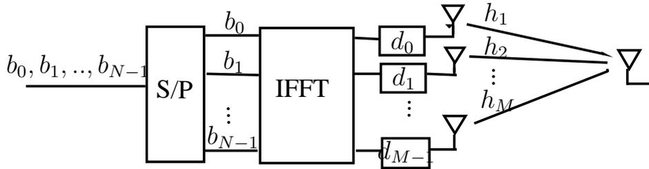
Figure 1.2: OFDM Block Diagram
