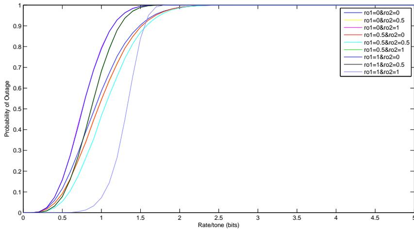
Figure 2.11: Two-user Gaussian interference channel with  $N=4$  and  $\text{SNR}=10\text{dB}$  (Frequency-selective)
