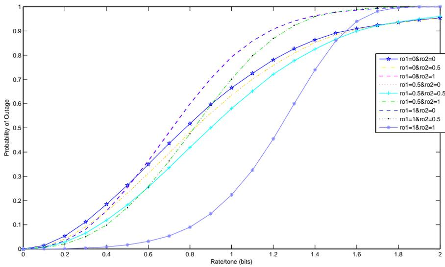
Figure 2.7: Two-user Gaussian interference channel with  $N=4$  and  $\text{SNR}=10\text{dB}$  (Frequency-flat)
