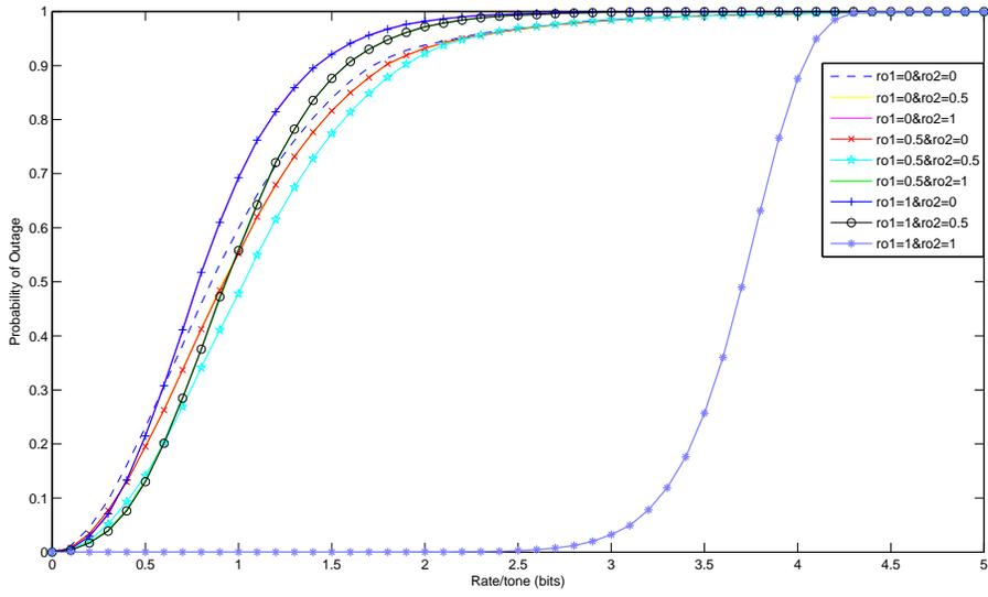
Figure 2.4: Two-user Gaussian interference channel with  $N=4$  and  $\text{SNR}=40\text{dB}$  (Frequency-flat)
