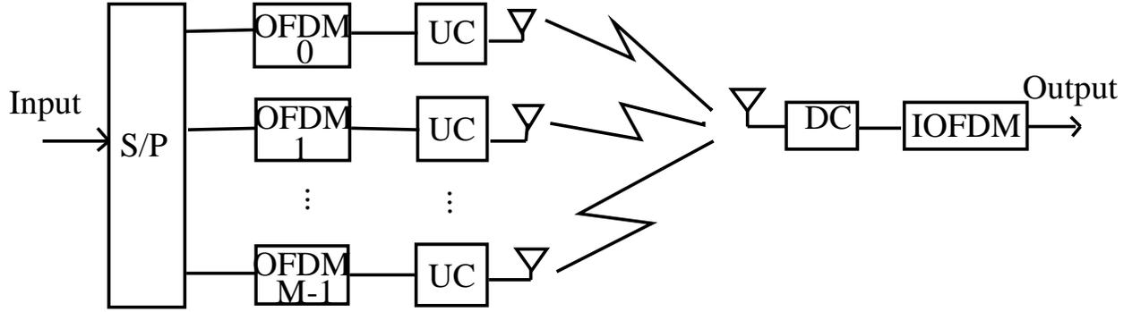
Figure 1.3: Subcarrier Diversity Block Diagram
