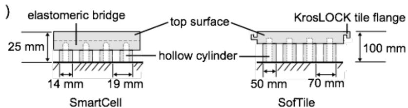
**Figure 1-7: Schematic representation of the buckling column designs of SmartCell (left) and SofTile (right) novel compliant floors**
