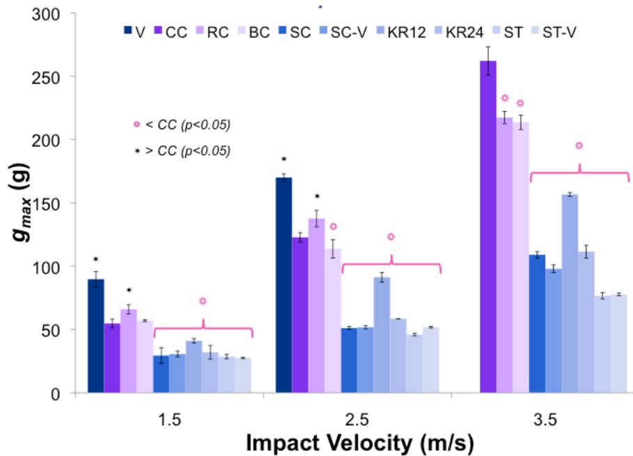
**Figure 2-4: Mean (SD) peak accelerations for impacts to the back of the headform at each impact velocity across all flooring conditions**
