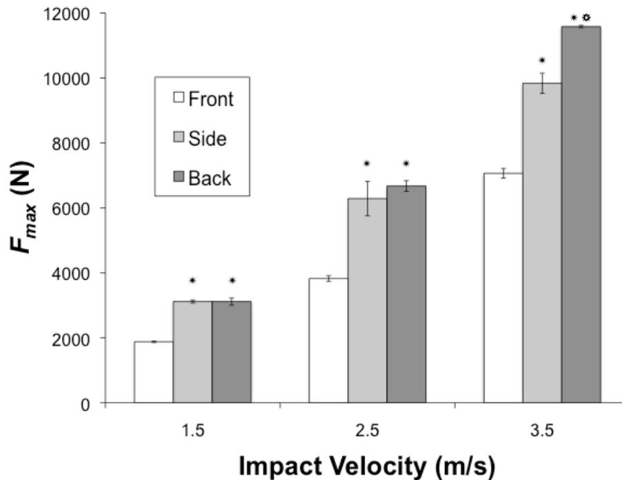
**Figure 2-3: Mean (SD) of peak force ( $F_{max}$ ) for impacts onto the front ( $F$ ), side ( $S$ ), and back ( $B$ ) of the surrogate headform at each impact velocity (testing completed on the control Commercial Carpet condition). \* indicates significant ( $p<0.05$ ) increase relative to  $F$ , \* indicates significant ( $p<0.05$ ) increase relative to  $S$ .**
