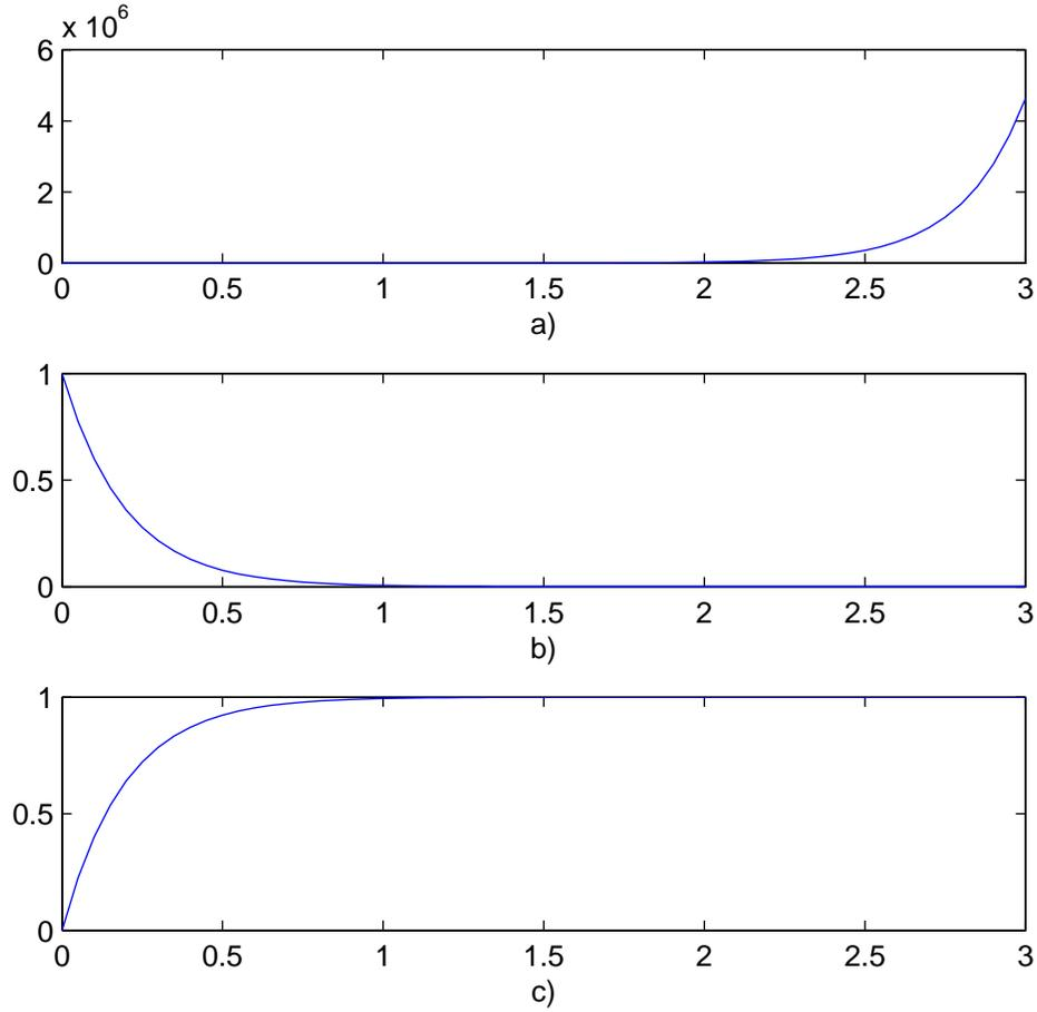
Figure 4.6. Curve fitting by Matlab for solving X term in the subthreshold triode region, a)  $X = \exp(V_{DS} / S_f)$ , b)  $X = \exp(-V_{DS} / S_f)$ , and c)  $X = 1 - \exp(-V_{DS} / S_f)$ .
