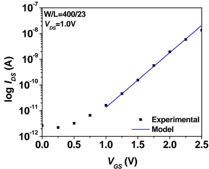
Figure 4.5. Comparison between modeling and experimental data for the subthreshold saturation region.
