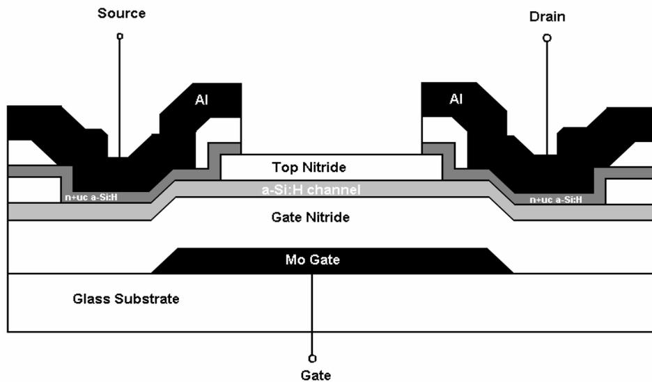
Figure 2.1. Cross-section of an inverted staggered a-Si:H TFT.
