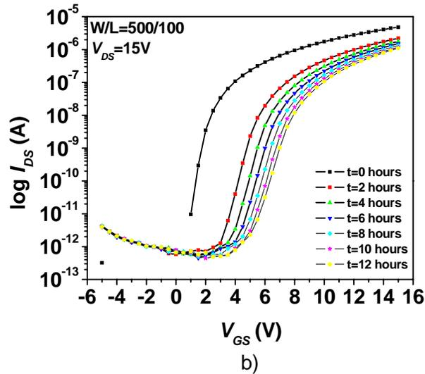
Figure 4.10. The change of Subthreshold slope in the presence of a) 20 V bias stress, b) 50 V bias stress.
