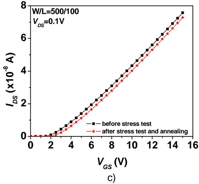
Figure 4.12. Comparison of annealed  $V_T$  before and after 12-hour stress tests for a) 10 V bias stress, b) 20 V bias stress, c) 50 V bias stress.
