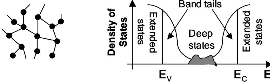
Figure 2.3. Atomic structure and DOS distribution in amorphous silicon.
