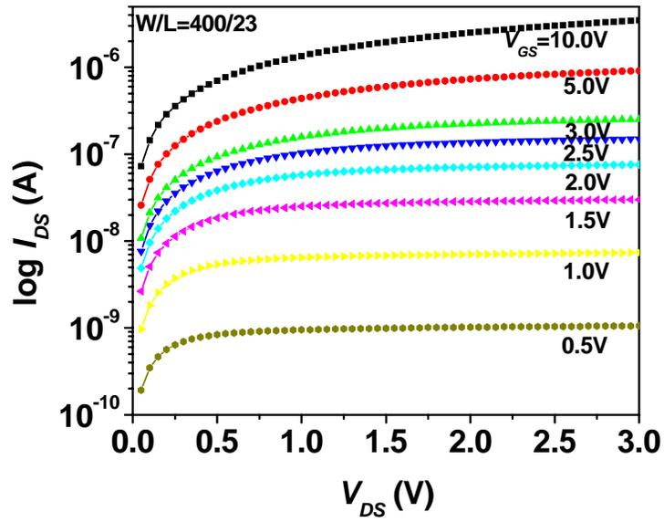
Figure 4.8.  $I_{DS}$  as a function of  $V_{DS}$  for different  $V_{GS}$  value.
