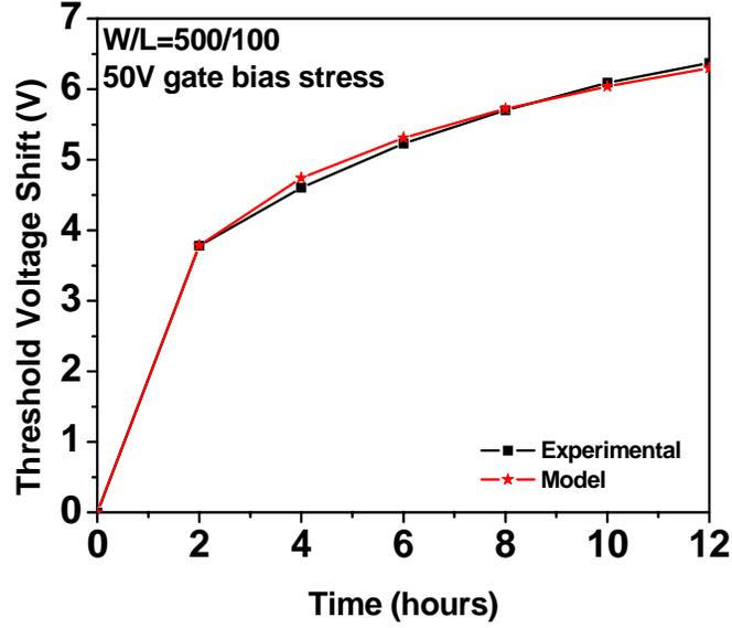
Figure 4.14.  $V_T$  shift as a function of stress time for a 12-hour, 50 V constant voltage stress test.
