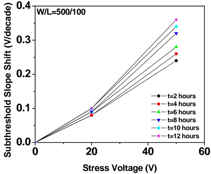
Figure 4.11. Subthreshold slope shift as a function of positive stress voltage for different stress times.
