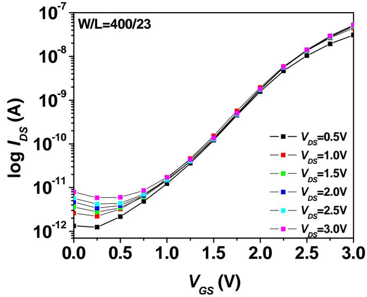
Figure 4.3.  $I_{DS}$  as a function of  $V_{GS}$  for different  $V_{DS}$  values.
