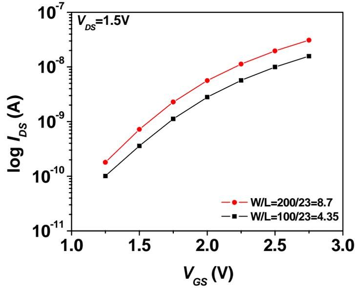
Figure 4.4.  $I_{DS}$  as a function of  $V_{GS}$  for different transistor dimensions.
