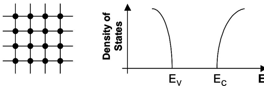
Figure 2.2. Atomic structure and DOS distribution in crystalline silicon.
