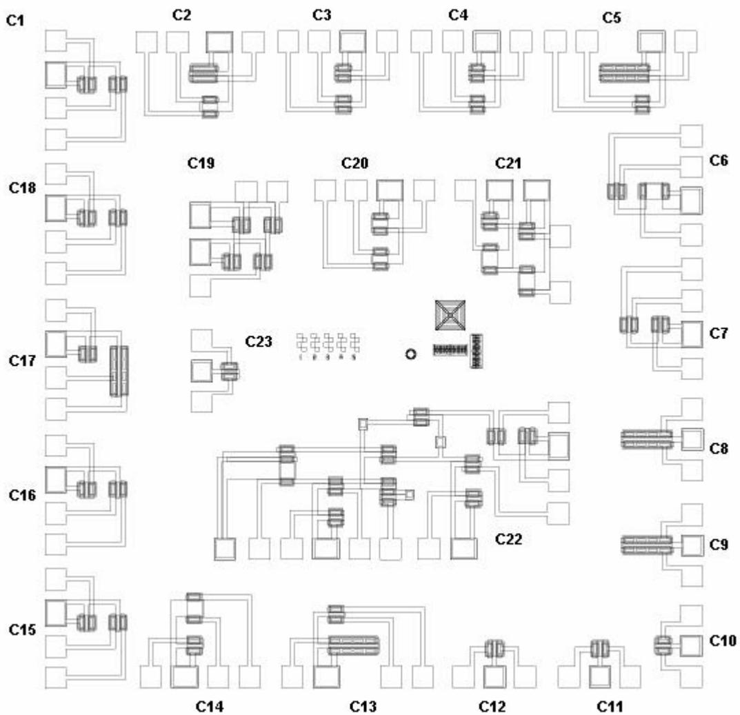
Figure C.1. Cadence layout of different current mirrors.
