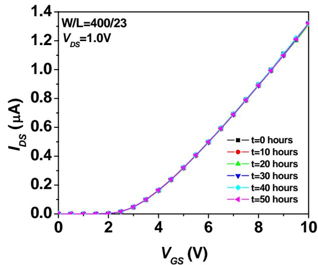
Figure 4.16. Threshold voltage characteristics under a 50-hour constant voltage stress in the subthreshold saturation region.
