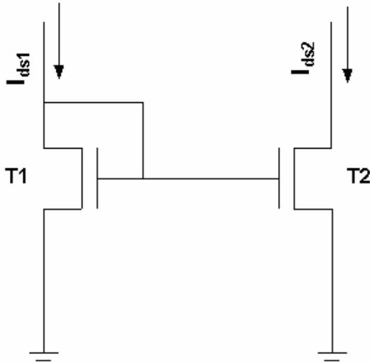
Figure 5.1. Schematic of a simple current mirror.
