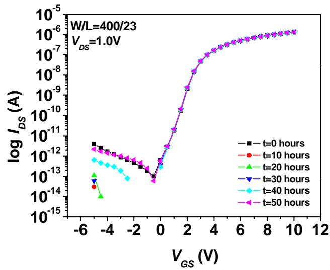
Figure 4.15. Subthreshold slope characteristics under a 50-hour constant voltage stress in the subthreshold saturation region.
