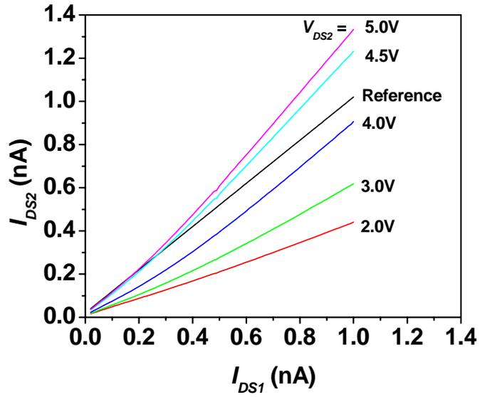
Figure 5.3.  $I_{DS1}$  versus  $I_{DS2}$  of the current mirror (65/23|65/23) on a die.
