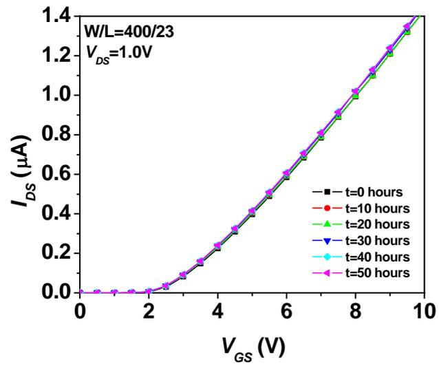
Figure 4.18. Threshold voltage characteristics under a 50-hour constant voltage stress in the subthreshold triode region.
