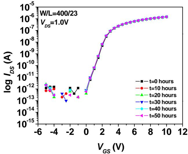
Figure 4.17. Subthreshold slope characteristics under a 50-hour constant voltage stress in the subthreshold triode region.
