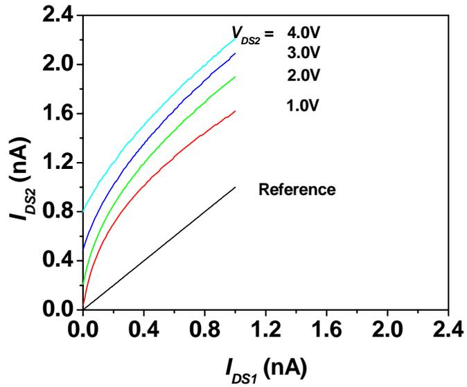
Figure 5.4.  $I_{DS1}$  versus  $I_{DS2}$  of the current mirror (65/23|65/23) on a packaged die.
