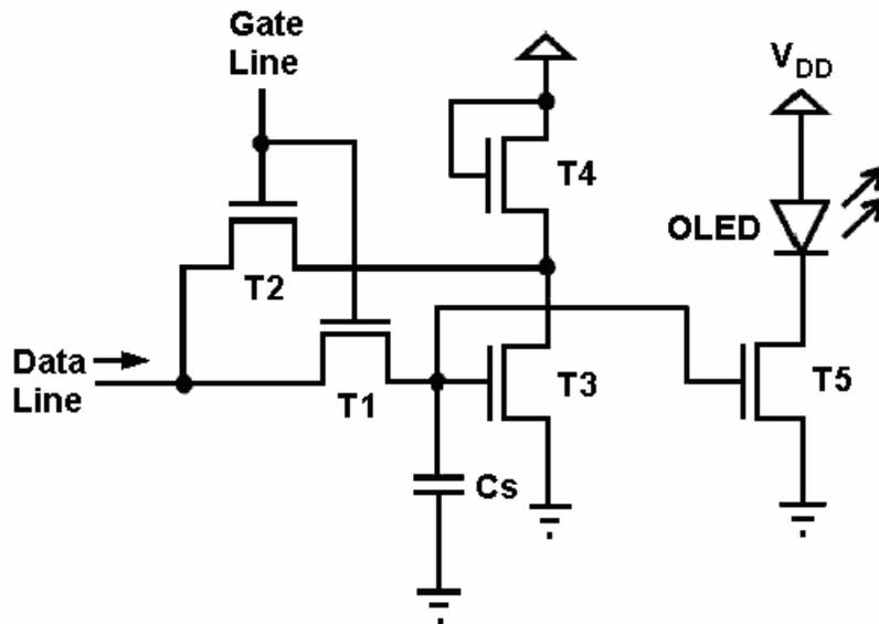
Figure 5.2. Schematic of a current-programmed pixel circuit.
