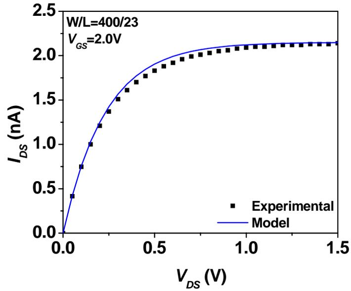
Figure 4.7. Comparison between modeling and experimental data for the subthreshold triode region.
