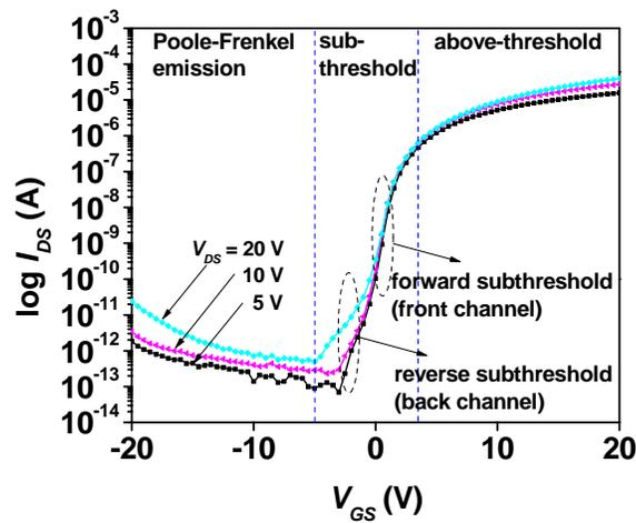
Figure 2.4.  $I_{DS}$  as a function of  $V_{GS}$  for different values of the drain-source voltage  $V_{DS} = 5, 10$  and  $20$  V showing the different regions of operations.
