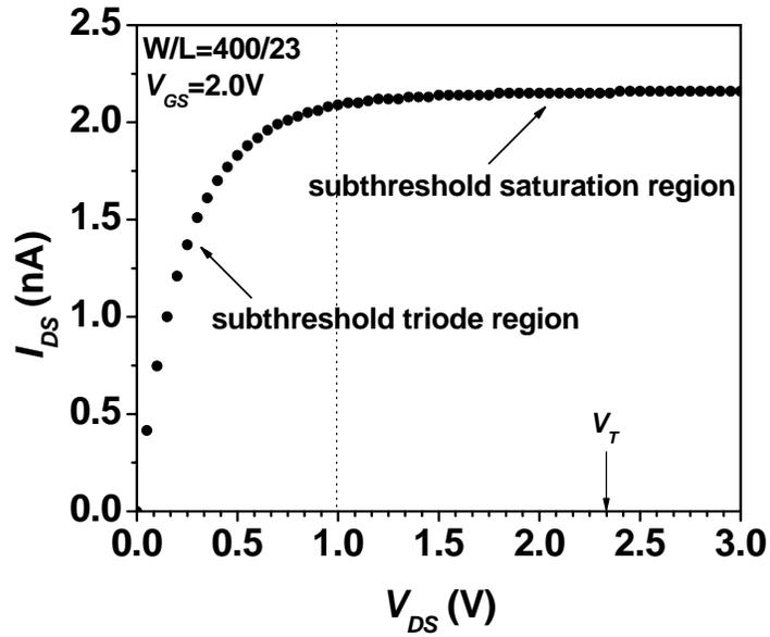
Figure 4.2.  $I_{DS}$  as a function of  $V_{DS}$  for a fixed  $V_{GS}$  value ( $V_{GS} = 2$  V).
