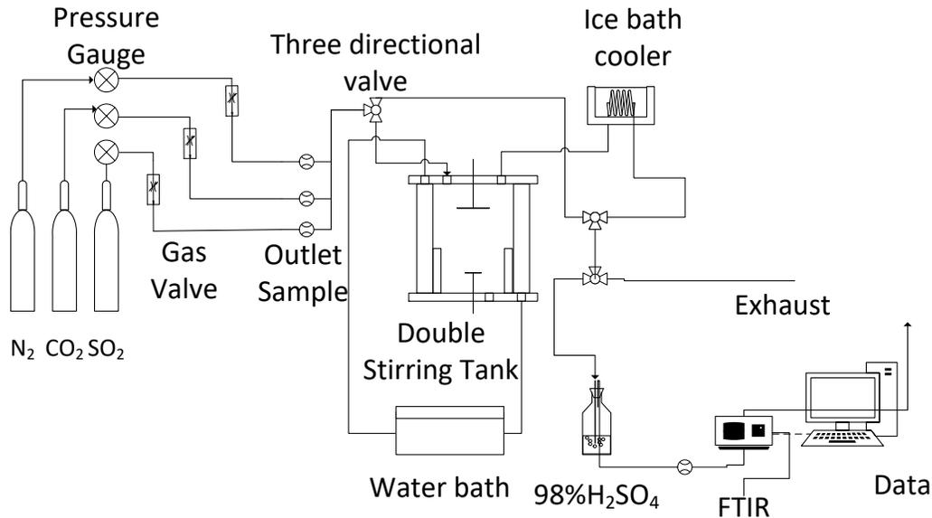
Figure 3-1. Experimental setup for the determination of mass transfer coefficient of CO<sub>2</sub> in aqueous ammonia
