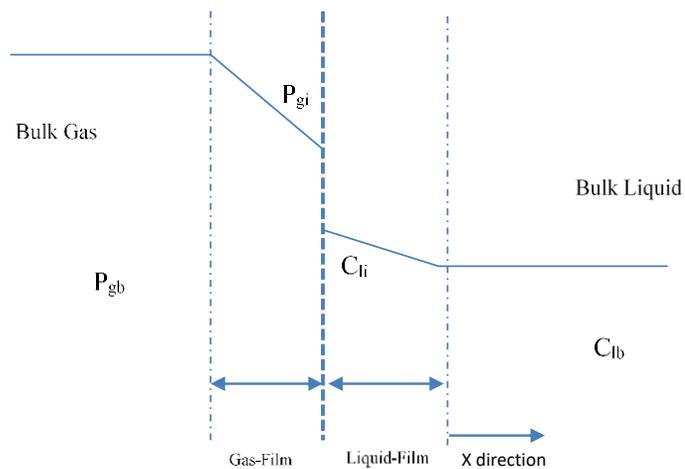
Figure 4-1 The diagram of two-film model
