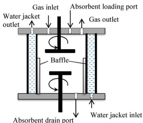
Figure 3-2 Diagram of double stirring tank
