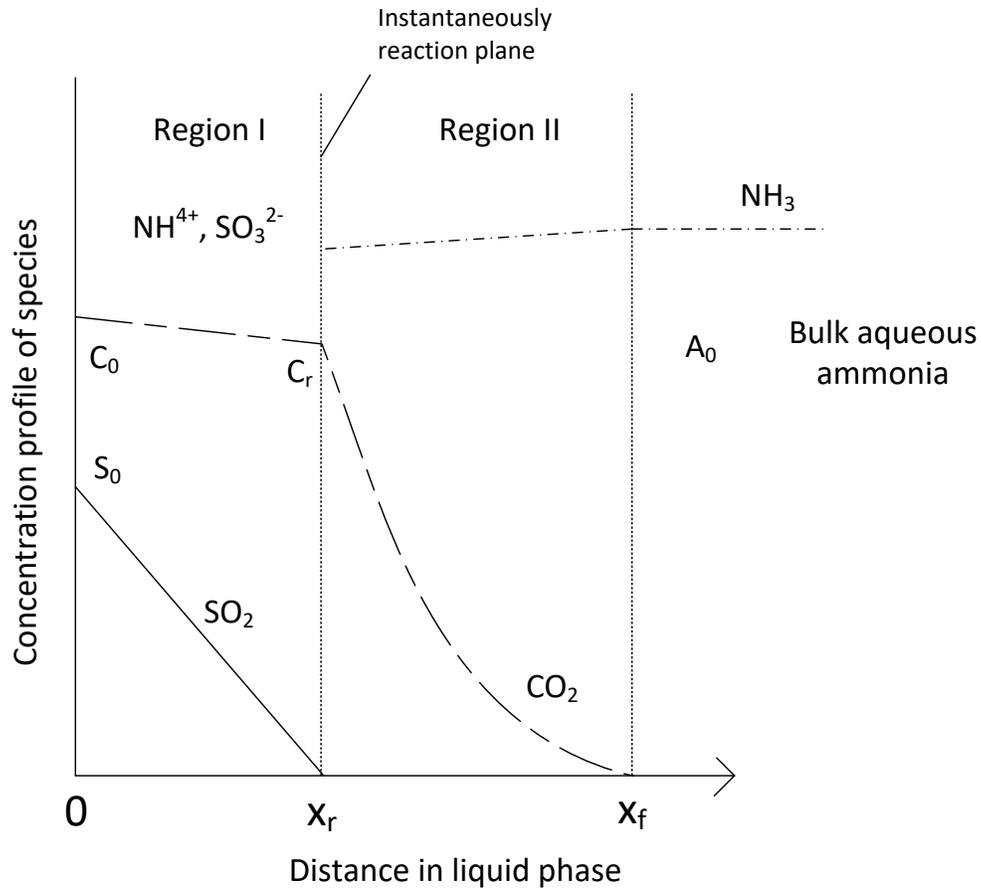
Figure 5-1 Diagram of concentration distribution of species in liquid phase
