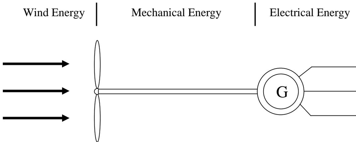
**Figure 2-1: Simplified Wind Generation Process.**
