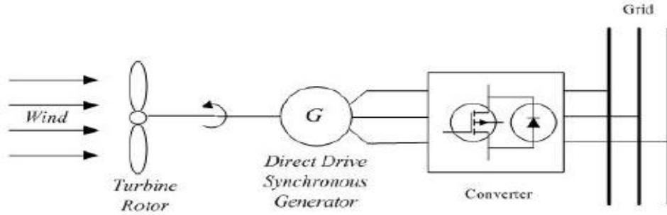
Figure 2-6: Type D - Variable Speed Wind Turbines with Full-Scale Frequency Converters [19].
