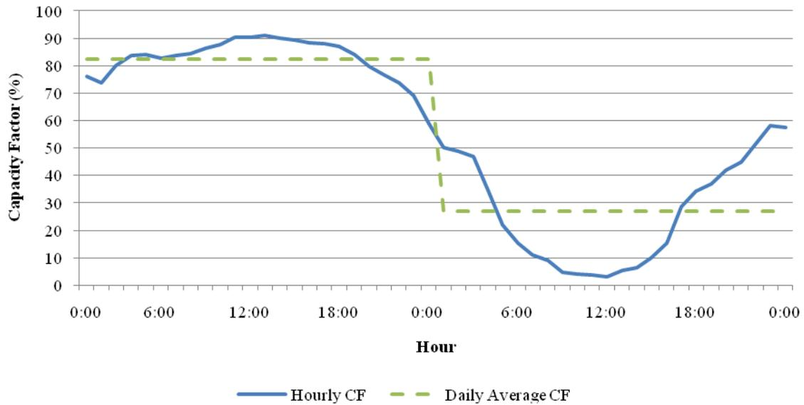
**Figure 3-11: Extreme Variation in Hourly Wind Generation CF: 23<sup>rd</sup> – 24<sup>th</sup> Nov 2010.**
