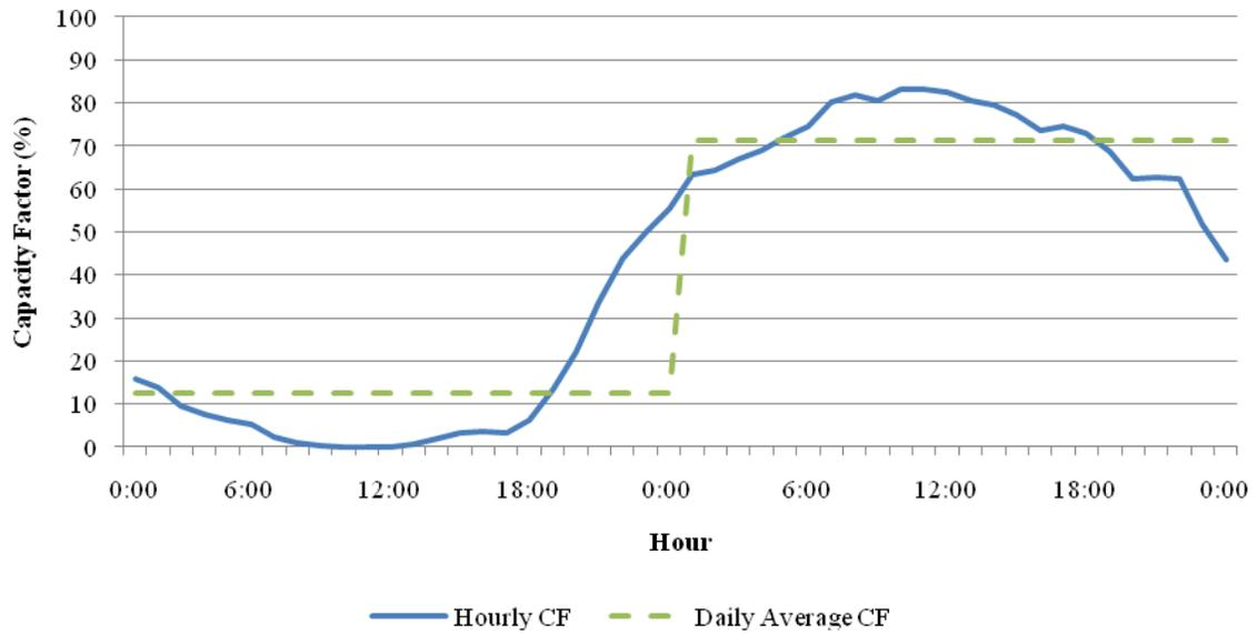
**Figure 3-9: Extreme Variation in Hourly Wind Generation CF: 29<sup>th</sup> to 30<sup>th</sup> Mar 2008.**
