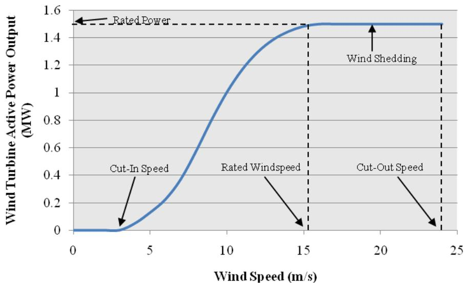
**Figure 2-9: Ideal Wind Turbine Power Curve.**
