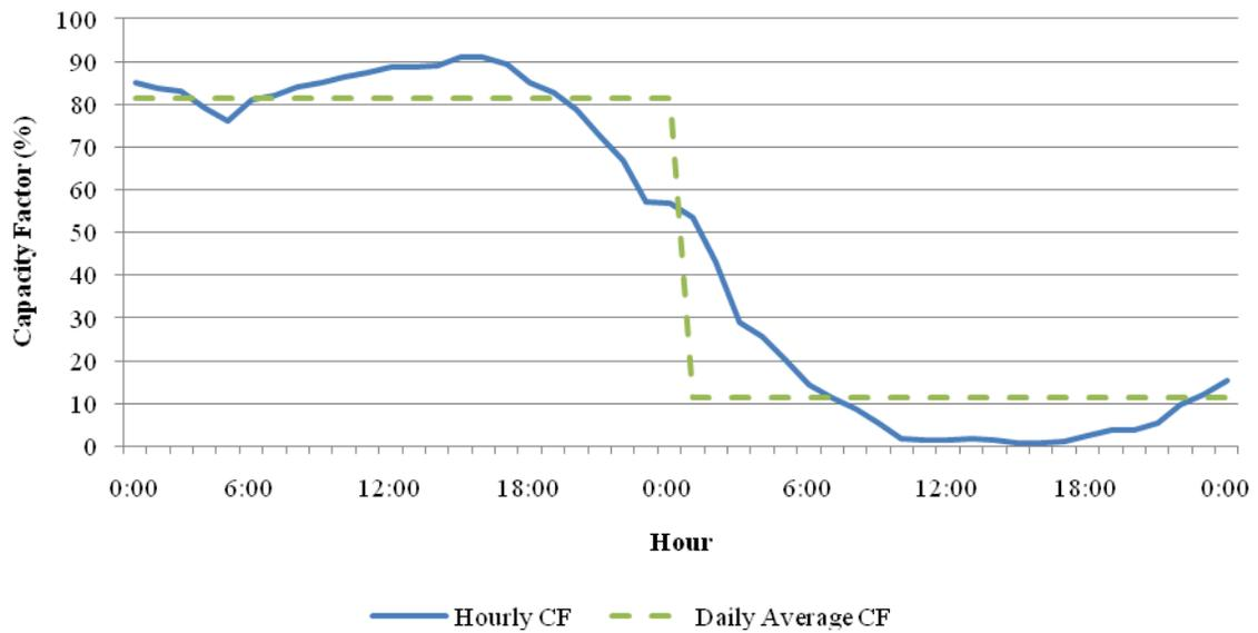
**Figure 3-10: Extreme Variation in Hourly Wind Generation CF: 31<sup>st</sup> Oct - 1<sup>st</sup> Nov 2009.**
