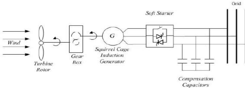
**Figure 2-3: Type A - Constant Speed Wind Turbines [19].**
