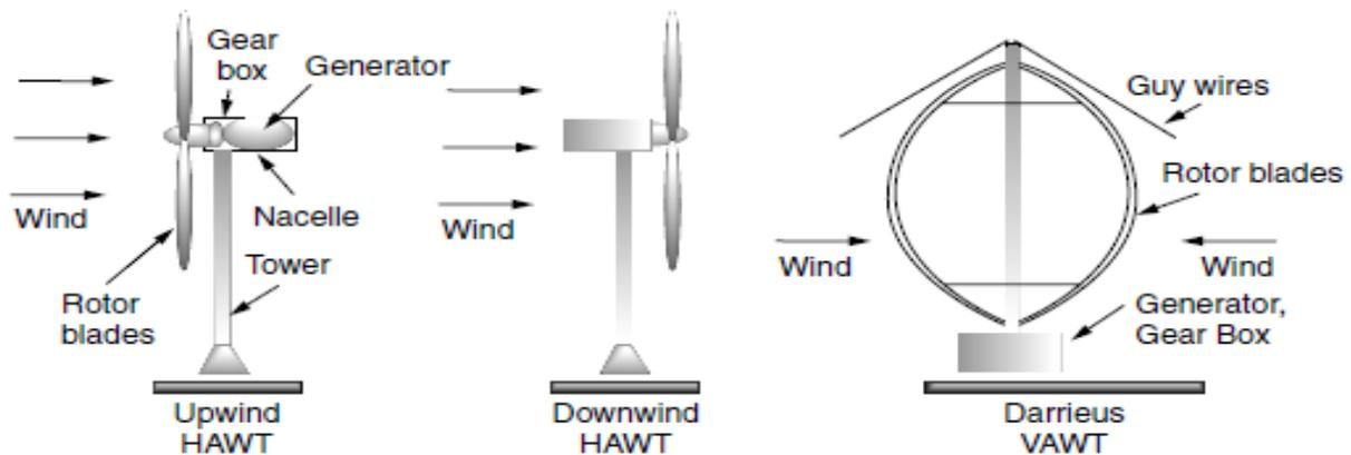
**Figure 2-2: Types of Wind Turbines [17].**
