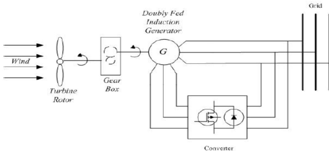
Figure 2-5: Type C - Variable Speed Wind Turbines with Partial Scale Frequency Converters [19].
