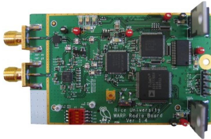
Figure 4.2: WARP Radio Board
