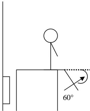
**Figure 4.1:** *Experimental Setup for Maximum Voluntary Exertion (MVE) Trial for Quadriceps. ( $0^\circ$  = leg in full extension)*
