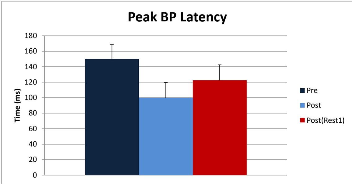
Figure 8a: Average (N=11) Peak BP latency at Cz electrode site across time. Peak BP latency determined as the total time difference between EMG onset and absolute peak BP.
