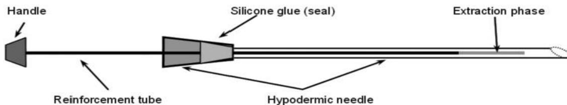
Figure 2: A special SPME device for *in vivo* extraction [5]
