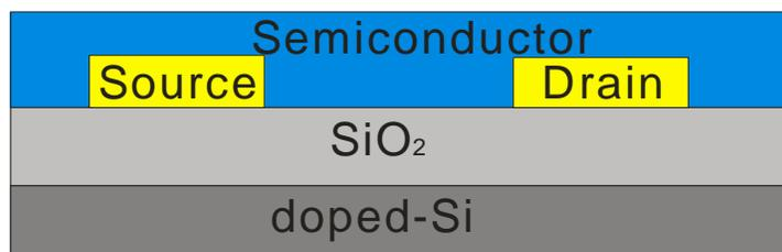
**Figure 3.1** Bottom gate, bottom contact structure of OTFT devices
