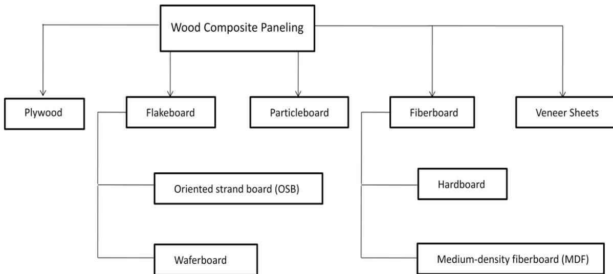
**Figure 6.1** Breakdown of the various types of composite panels available (Binggeli, 2008; Rivela et al, 2007)
