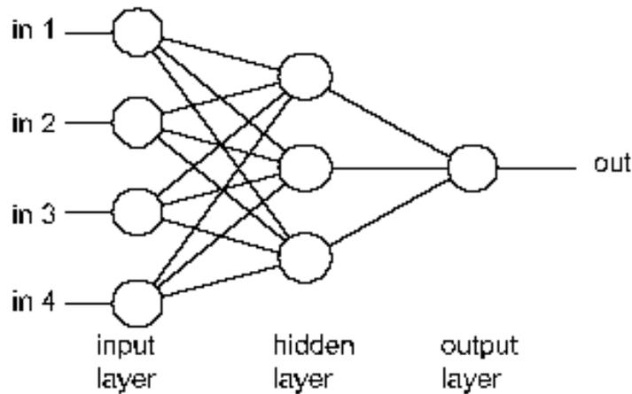
**Figure 4.7: Artificial Neural Network Architecture (source: [www.imtech.res.in](http://www.imtech.res.in))**
