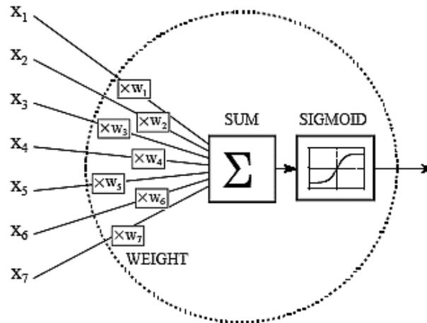
**Figure 4.8: Neural Network Active Node (source: [www.dspguide.com/ch26/2.htm](http://www.dspguide.com/ch26/2.htm))**
