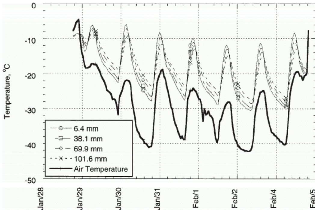
**Figure 2.2: Pavement and air temperature profile over time (Source: Bosscher et al., 1998)**
