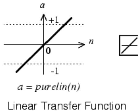
**Figure 4.11: A Typical Linear Transfer Function (source: [www.mathworks.com](http://www.mathworks.com))**
