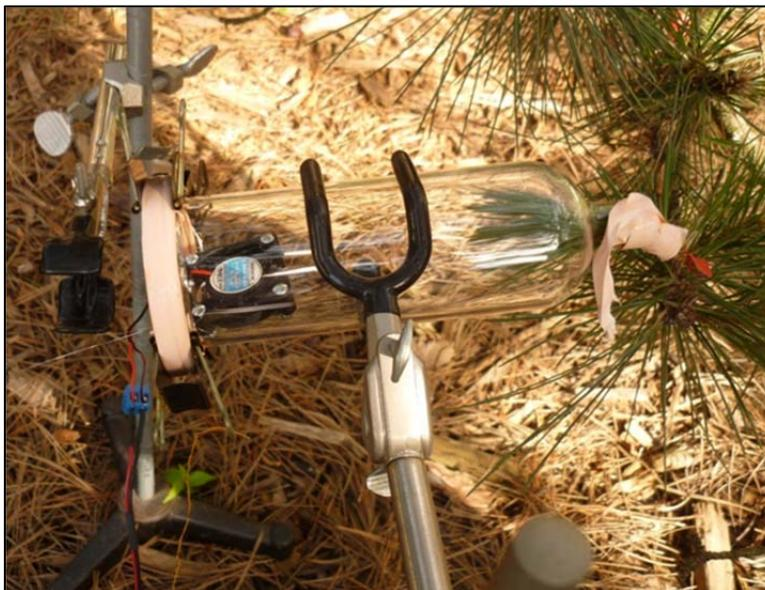
**Figure 3-3.** Experimental setup for on-site sampling of biogenic emissions.
