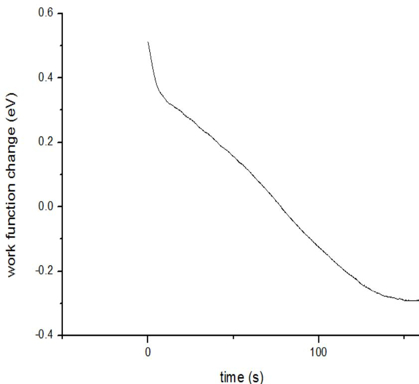
Figure 3-7 Work function change of a 30-ML ice film with freshly deposited potassium when  $\text{CCl}_4$  gas is introduced into the vacuum chamber at  $5 \times 10^{-8}$  torr for 150s.
