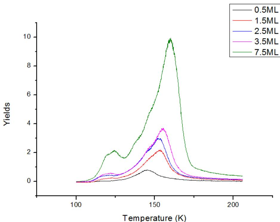
Figure 3-2 TPD spectrum of H<sub>2</sub>O with QMS filament 1.0mA.
