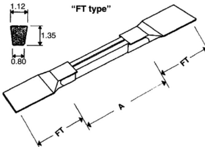
Figure 2-3 Sketch of the SAES getter (potassium dispenser). FT = terminal length = 10mm; A = active length = 17mm.<sup>79</sup>
