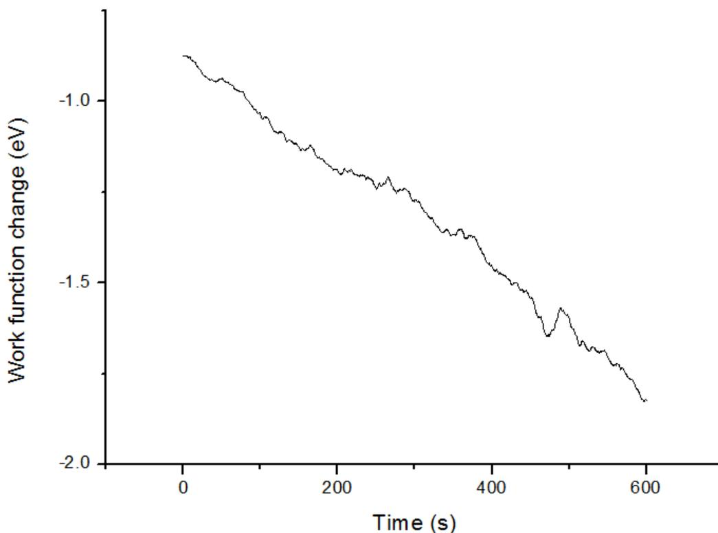
Figure 3-9 Work function change measurement of a potassium-deposited ice film during  $\text{CCl}_4$  exposure for 10 minutes at 100K.
