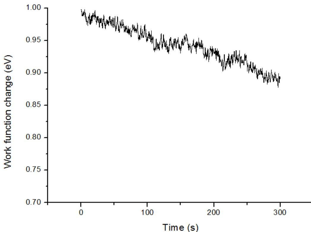
Figure 3-6 Work function change of a 30-ML ice film (no potassium deposition) when  $\text{CCl}_4$  gas is introduced into the vacuum chamber at  $5 \times 10^{-8}$  torr for 5 minutes.
