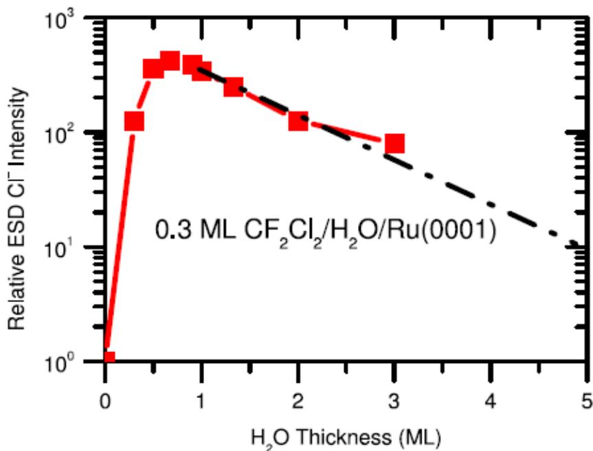
Figure 1-2 Relative Cl<sup>-</sup> yields desorbing from 250eV primary electrons incident onto 0.3 ML CF<sub>2</sub>Cl<sub>2</sub> adsorption on top of H<sub>2</sub>O-precovered Ru substrate varying with H<sub>2</sub>O spacer thickness. The dash-dot line is to extrapolate the Cl<sup>-</sup> yield to the 5 ML H<sub>2</sub>O spacer.<sup>27</sup>
