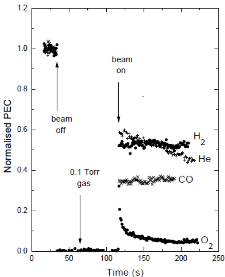
Figure 1-8 Photoemission current before and during exposure to 0.1 torr of different gases.<sup>7</sup>
