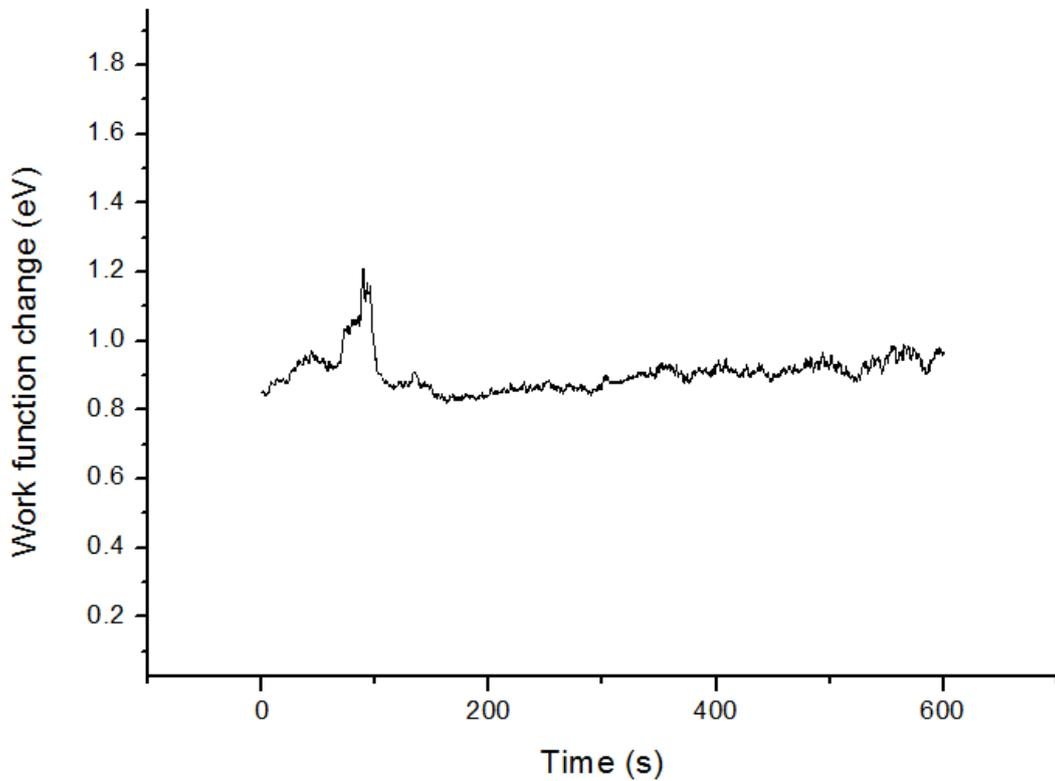
Figure 3-5 Work function change for a 15-ML ice film with freshly deposited potassium after heating to 168 K, measured as a function of cooling time (10 minutes).
