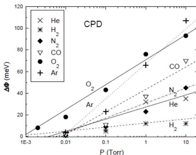
Figure 1-7 Work function changes with different exposure pressures.<sup>7</sup>
