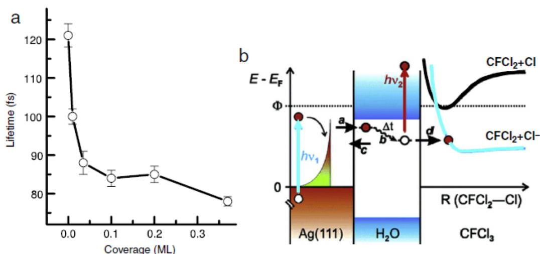
Figure 1-3 (a) Lifetime of the pre-solvated electrons as a function of the coverage of  $\text{CFCl}_3$  adsorbed on 5 ML  $\text{H}_2\text{O}/\text{Ag}(111)$ . (b) Schematic diagram for the life cycle of the photoinjected electrons in  $\text{CFCl}_3 / \text{H}_2\text{O} / \text{Ag}(111)$ : photoinjection of electron into the loosely bound  $e_{\text{pre}}$  state residing below the vacuum level(a); solvation in the ice layer (b); back
