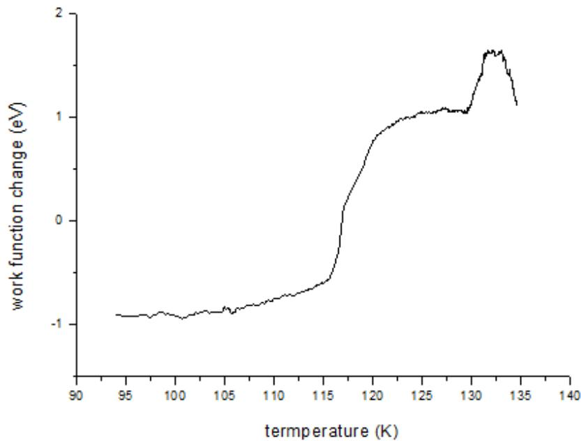
Figure 3-3 Work function change for a 15-ML ice film with freshly deposited potassium, measured as a function of temperature. The current of heating filament was 0.8 A.
