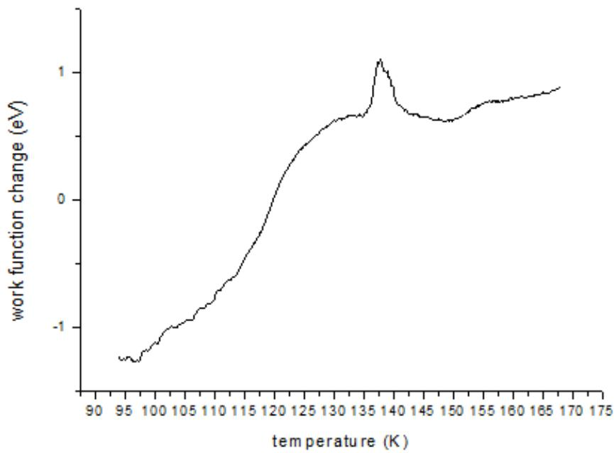
Figure 3-4 Work function change for a 15-ML ice film with freshly deposited potassium, measured as a function of temperature. The current of heating filament was 1.0A.
