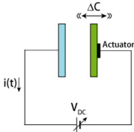
Figure 2-2 Schematic diagram of Kelvin probe. The blue plate is the sample and the green plate is the probe mesh.<sup>78</sup>
