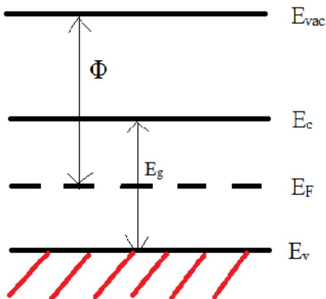
Figure 2-1 General band and diagram with the vacuum level  $E_{vac}$ , the conduction band  $E_c$ , valence band  $E_v$ , band gap  $E_g$ .
