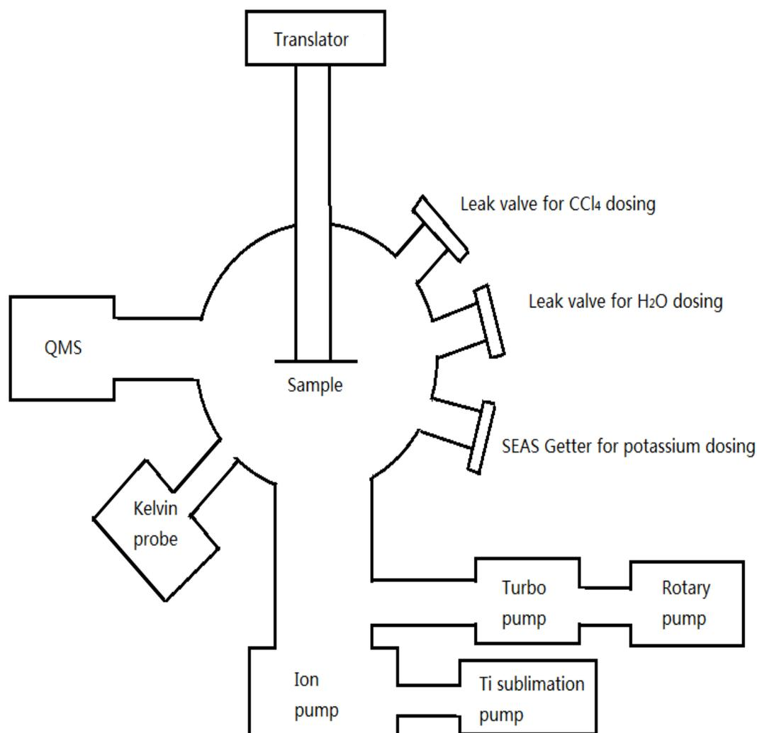
Figure 2-4 Schematic diagram of the UHV system.
