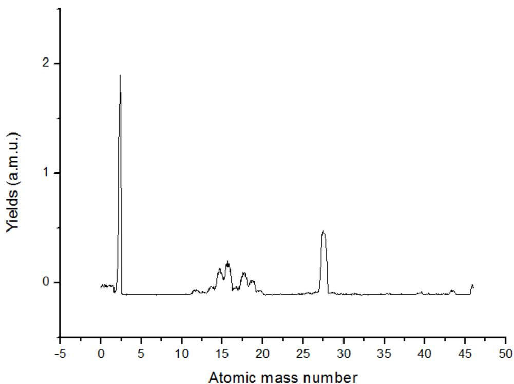
Figure 3-1 QMS scan of background gases with filament 1.5mA.
