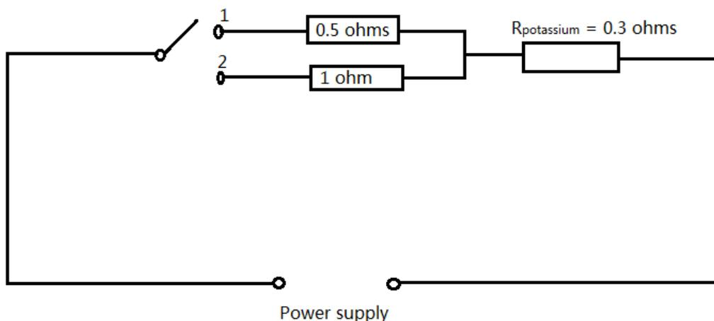
Figure 2-5 Schematic diagram of the control circuit. Position 1 for dosing potassium atoms and 2 for degassing.
