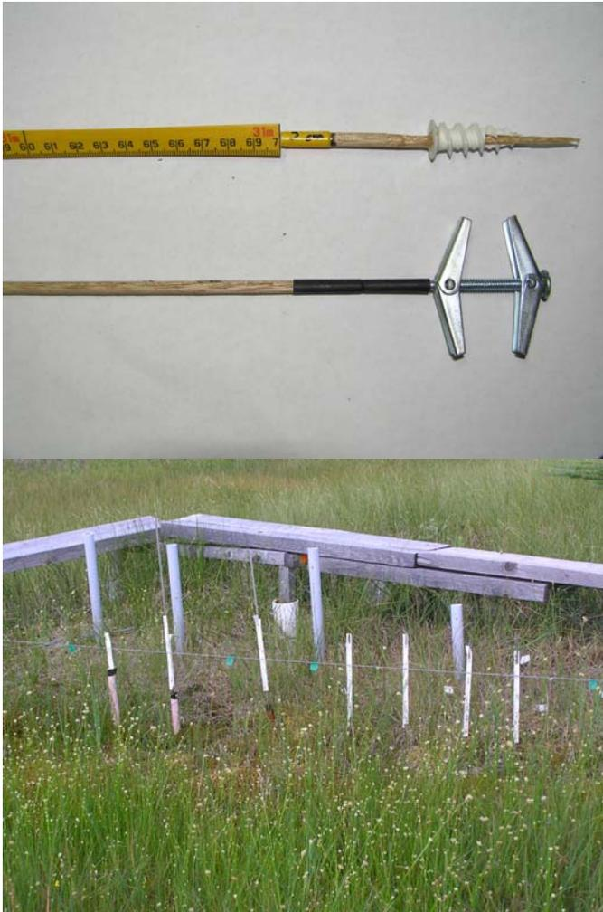
**Figure 3.2 Top: Shallower (5 cm) squishometer (upper) and deeper squishometer (lower) prior to installation; Bottom: Squishometers installed at the Experimental South site (note use of white measuring tape, opposed to yellow).**
