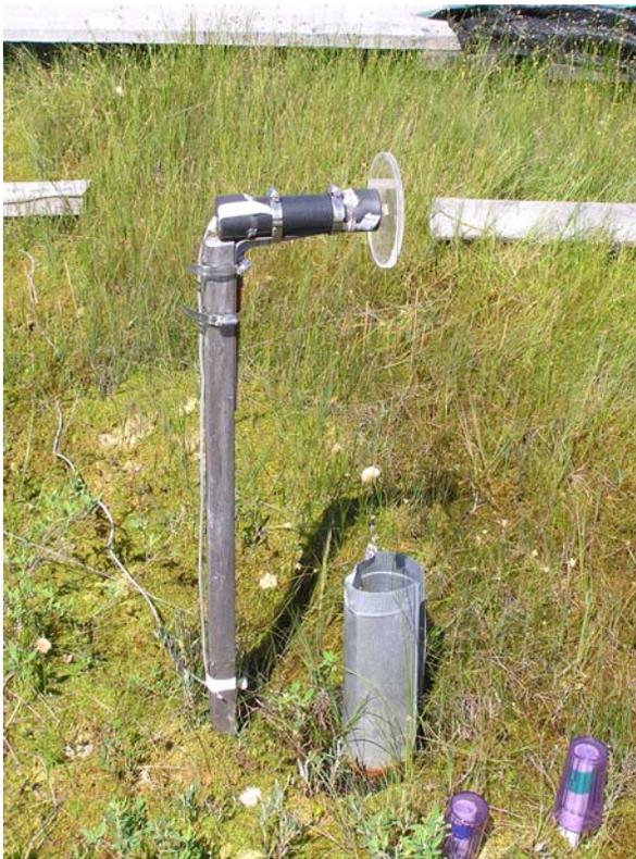
Figure 3.3 Float-pulley system measuring the Control lawn water table.
