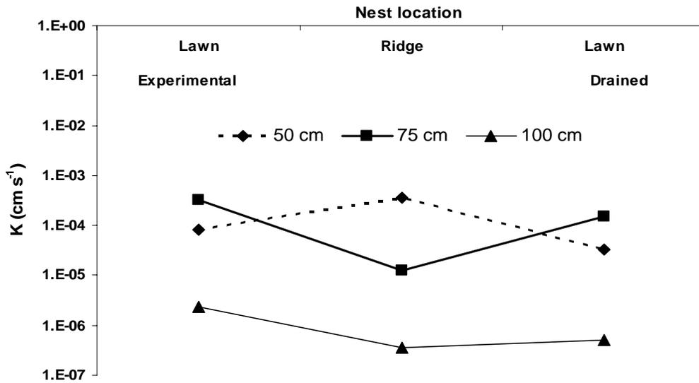
Figure 4.10 Hydraulic Conductivity through the EDZ transect
