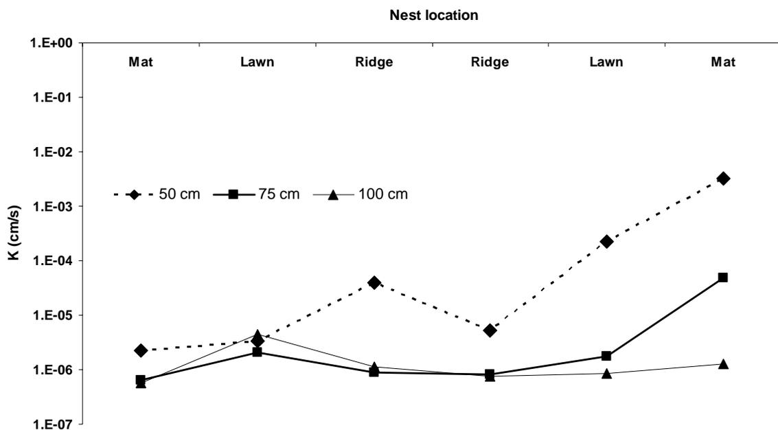
Figure 4.11 Hydraulic Conductivity through the DDZ transect
