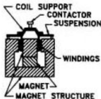
**Figure 3: A voice-coil transducer. Image source: Cholewiak and Wollowitz (1992).**
