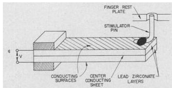
**Figure 6: A piezoelectric transducer. Image source: Bliss et al. (1970).**
