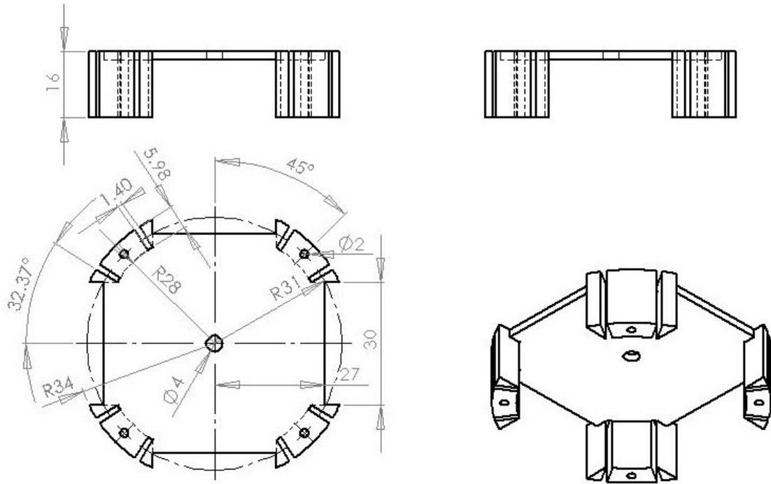
**Figure 27: CAD drawing of top part of PVC disk for soft shell prototype.**
