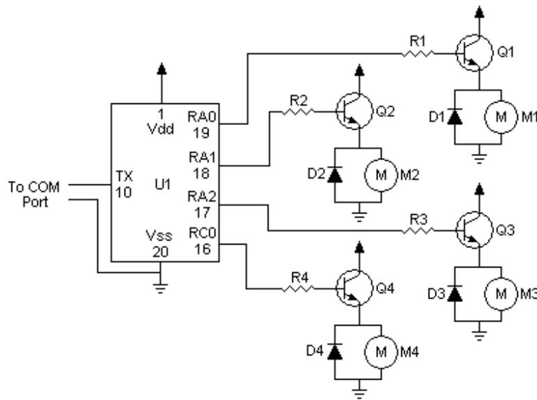
**Figure 22: Tactor control circuit.**
