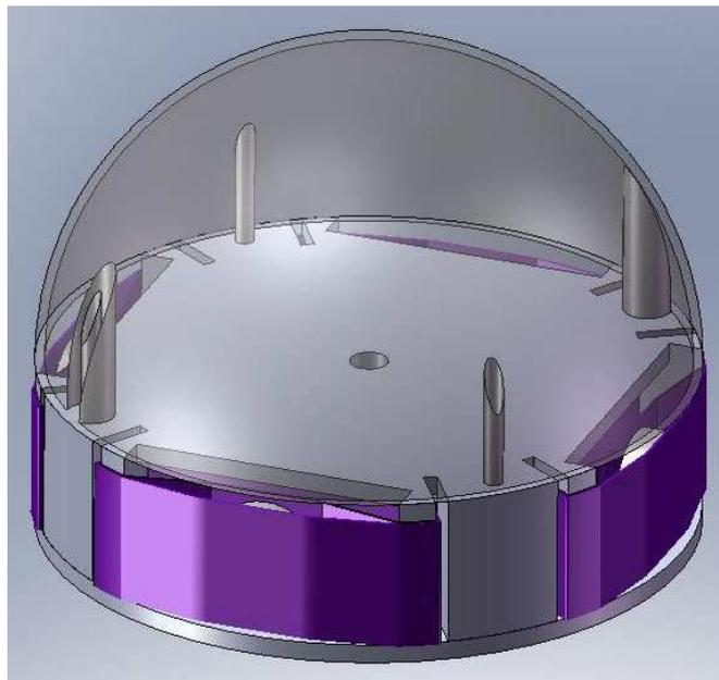
**Figure 21: Soft shell prototype (not shown: wires).**
