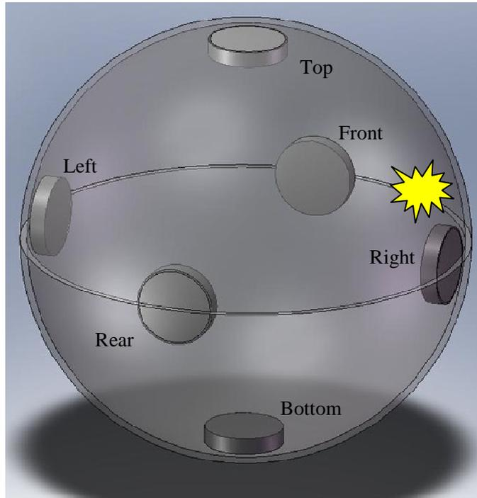
**Figure 25: Collision occurring midway between the front and right factors.**
