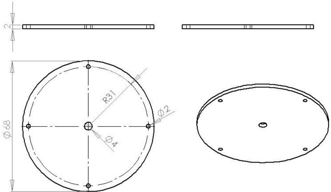
Figure 28: CAD drawing of bottom part of PVC disk for soft shell prototype.
