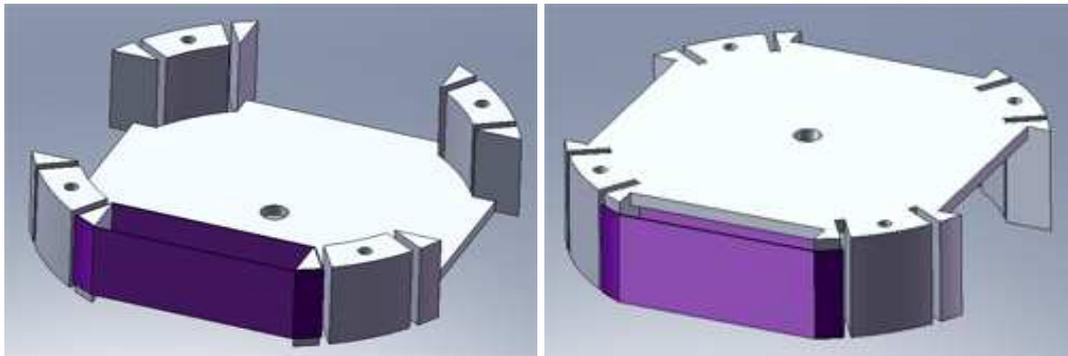
**Figure 19: PVC disk for the soft shell design. The disk on the right is inverted to show bottom details.**
