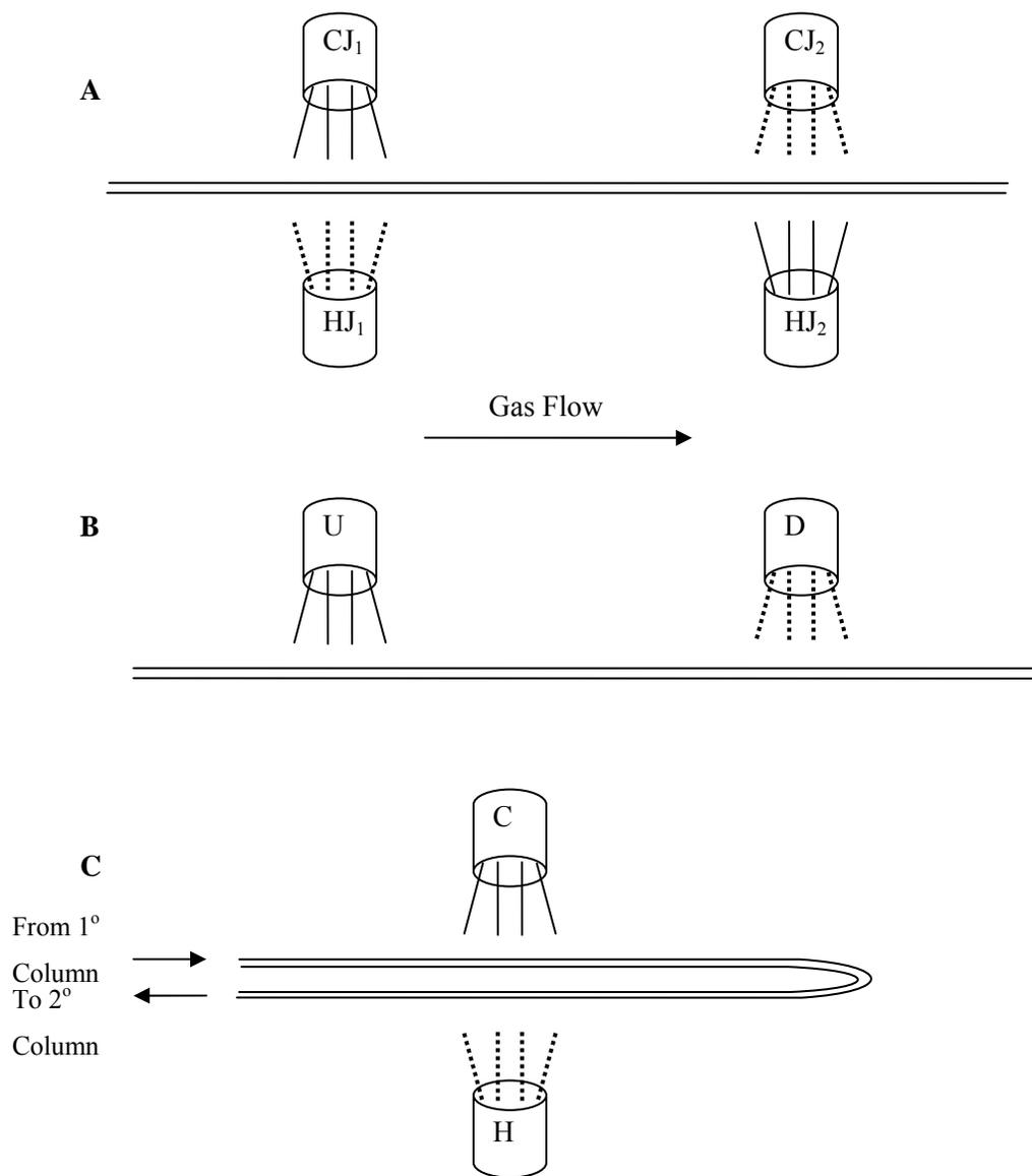
**Figure 1-7:** Block diagrams of dual stage cryogenic interfaces with no moving parts. (A) Alternating cryogenic jets ( $CJ_1$  and  $CJ_2$ ) for analyte trapping with hot air jets ( $HJ_1$  and  $HJ_2$ ) for re-mobilization.<sup>16</sup> (B) Beens' modulator using two cryojets with band remobilization at the oven temperature.<sup>18</sup> (C) With the addition of the delay loop, only one alternating cryogenic jet and hot jet are required.<sup>19</sup>
