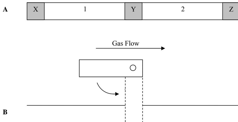
**Figure 1-5:** Block diagrams of the thermal based modulators designed by Phillips et al. (A) The dual-stage interface with resistive heating,<sup>12</sup> and (B) the rotating thermal modulator that provided approximately 100°C increase of temperature above the oven temperature.<sup>13,14</sup>
