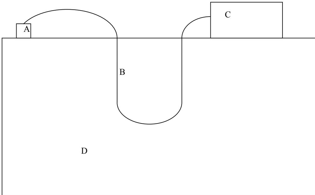
**Figure 5-2:** Experimental setup for flow rate of the modulator: A inlet, B modulator, C flowmeter, D oven.
