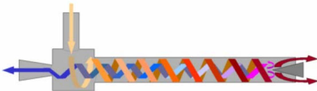
**Figure 1-8:** Vortex cooler. Red arrows indicate high kinetic energy air molecules, while the blue arrows indicate low kinetic energy air molecules.<sup>28</sup>
