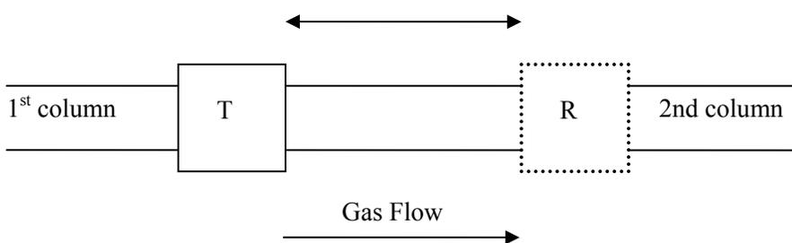
**Figure 1-6:** Longitudinally modulated cryogenic system (LMCS)<sup>15</sup>
