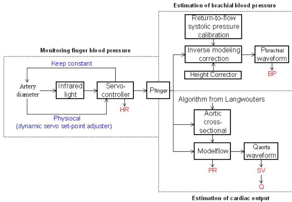
**Figure 4: Schematic Representation of the Finometer™ Layout**
