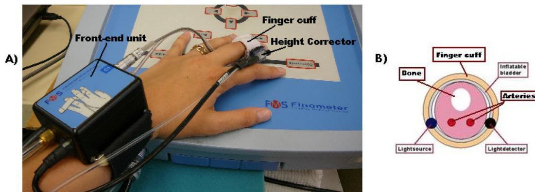
**Figure 5: A) Finger Cuff; B) Finger Cross-Section** [Modified from FMS website]
