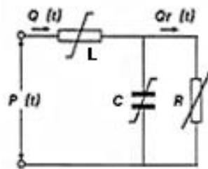
**Figure 30: Electric circuit representing the modelflow model** [modified from FMS website]
