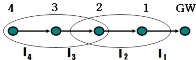
Figure 4.1: Interference range in a chain
