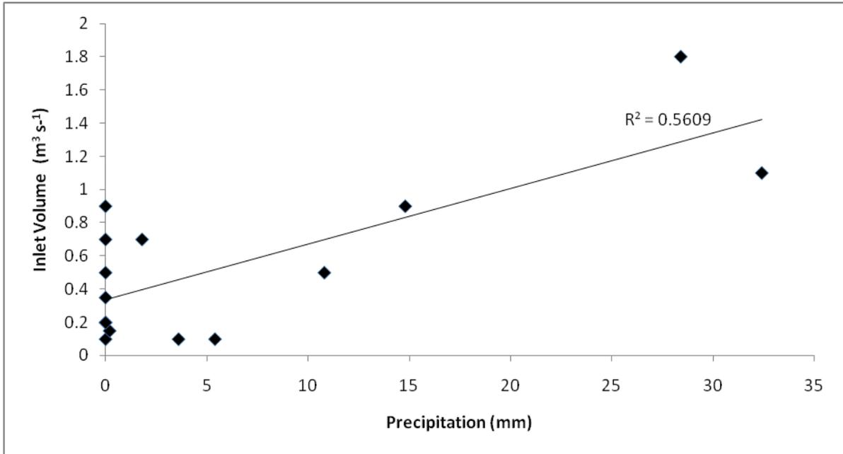
Figure 3a: The relationship between precipitation and inflow water volume for Columbia Lake inflow in 2007, calculated from area velocity method by H. Yu 2007.
