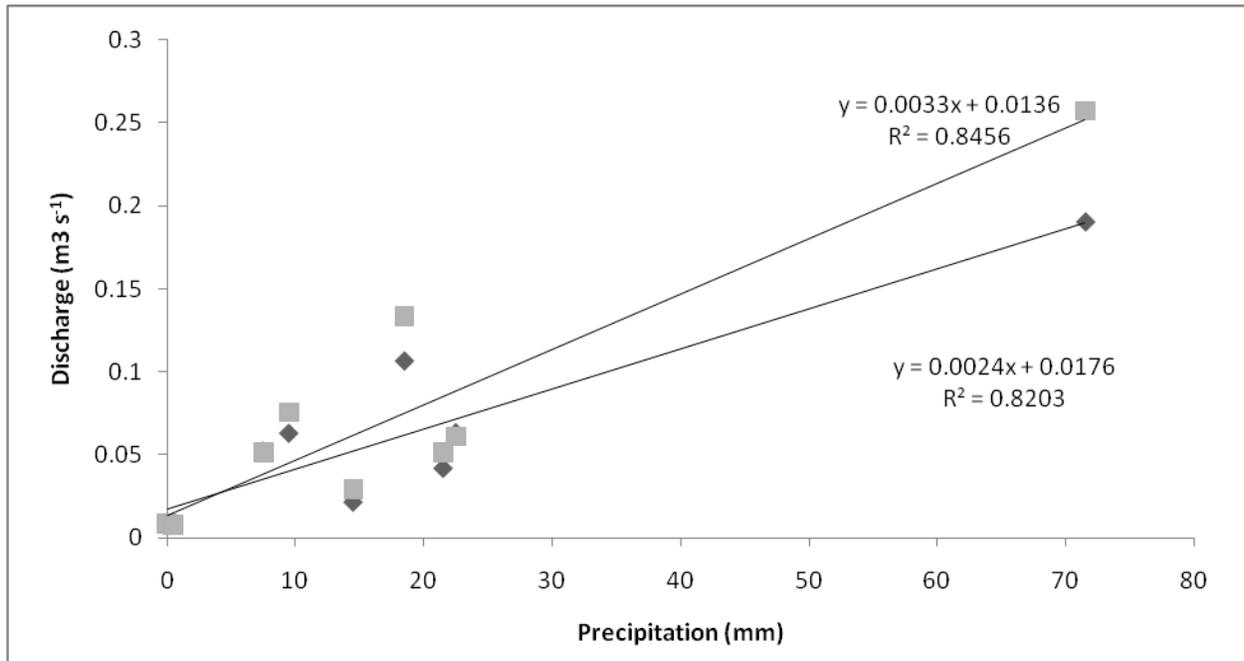
Figure 4: Relationship between Clair Lake inflow and outflow water volume with precipitation for 2009, diamond=inflow and square=outflow, this was used to estimate flow characteristics for 2007 and 2008.
