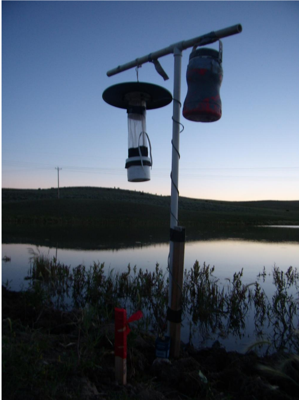
Figure 1: Image of adult mosquito night traps used to collect tissue samples around treatment and control reservoirs during the 2013 field season. Night traps utilized a dry ice container which gradually released CO 2 into the immediate atmosphere as an attractant to adult mosquitoes. Individuals drawn in to the trap were blown by an electric fan into a sampling net.
