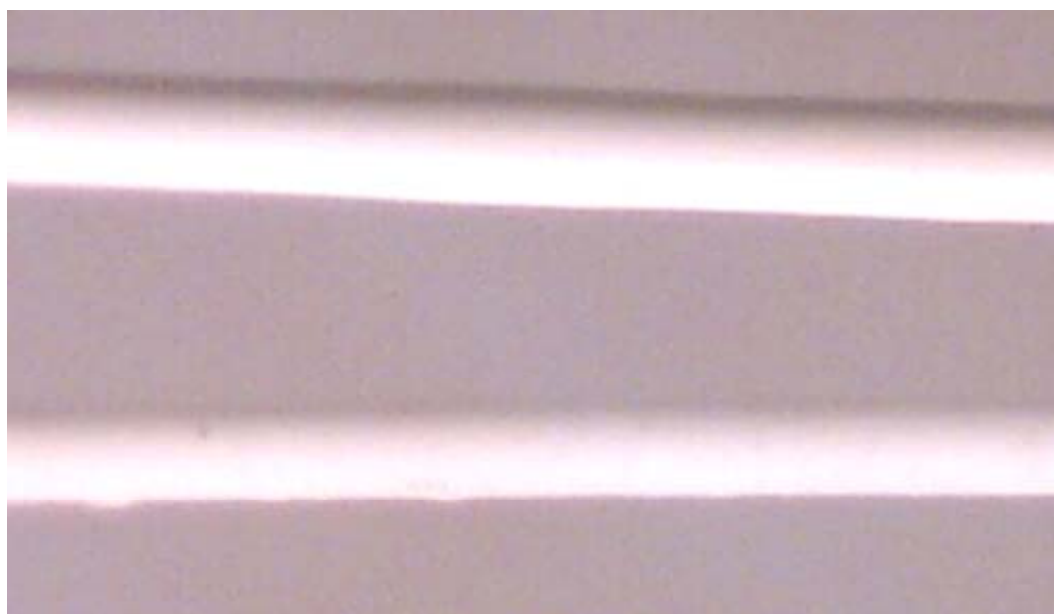
Figure 2-6. Fiber with PAN membrane (top) and original fiber before coating (bottom).
